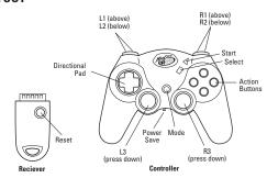
**Antenna Receiver:** Used to transmit and receive data from the controller to the game console.
