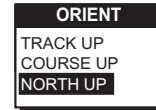
Figure A. You can choose from TRACK UP (direction you are moving at the top of the screen), COURSE UP (destination of the current leg at the top of the screen) and NORTH UP (north at the top of the screen).
