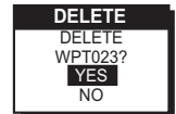
Figure D. This screen prompts you to select YES or NO in deleting the waypoint named.
