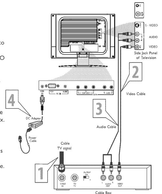
The AUDIO and VIDEO In jacks on the rear of the LCD TV enable quick connections of other equipment. Connect a VCR, DVD Player, Video Game, Camcorder, etc., to these jacks. To view the material playing on the other equipment, set the LCD TV to its AV Mode.
