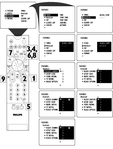
To block all channels at once, highlight ALL in the channel list. Then press the CURSOR RING RIGHT to block, Remove the blocks the same way.
