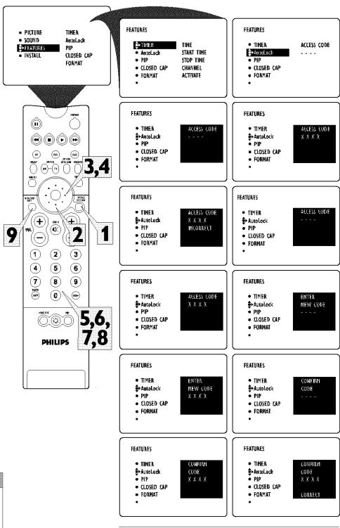
You can also set up a new access code from the main AutoLock™ Submenu using the SETUP CODE option. Simply enter and confirm the new Code to activate it.
