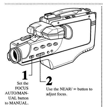
Your camcorder will focus automatically on the subject in the center of the EVF (even when you are zooming in and out) when the FOCUS AUTO/ MANUAL switch is set to AUTO. However, we recommend that you focus the camcorder manually under certain conditions – specifically, when filming:
