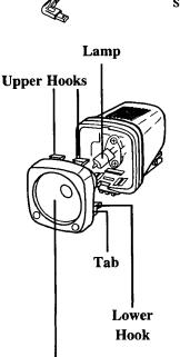
To remove the front case, press and hold the tab, then slide off the front case.
