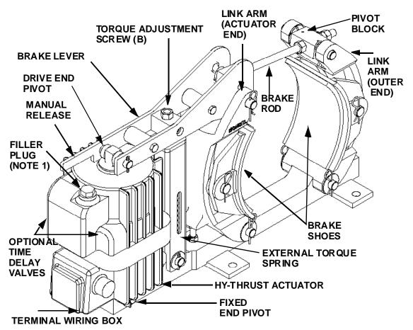
NOTE 1: FILL TO LOWER RIM OF FILLER HOLE. USE ONLY FLUID IDENTIFIED ON THE ACTUATOR NAMEPLATE. DO NOT OVER-FILL
