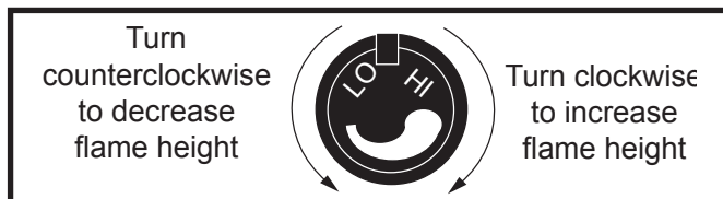
Fig. 42 Flame adjustment knob for Honeywell valve.
