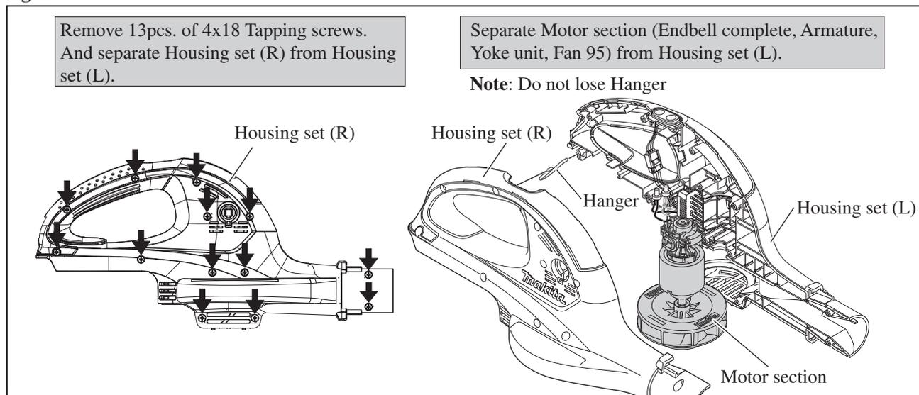
(3) Fan 95 and Armature can be replaced as illustrated in **Fig. 3**.
