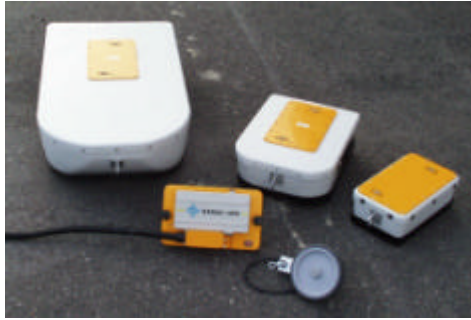
Figure 5.1 From left to right: Shielded 250, 500 and 800 MHz antennas. In front: electronics unit and survey wheel.
