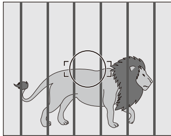
❷ Two or more objects overlap at different distances within the focus frame (animals in cages, etc.)
