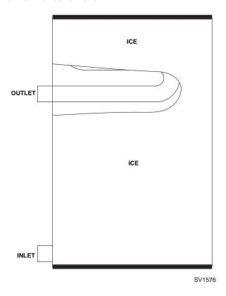
Figure 7-8. Extremely Thin Ice Formation at Evaporator Outlet
