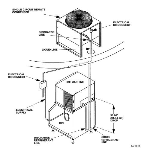
Figure 2-10. Typical Single Circuit Remote Condenser Installation
