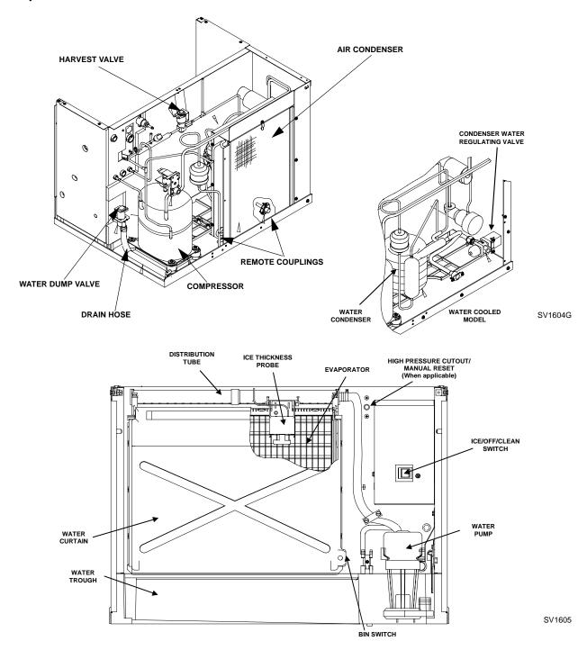
Figure 3-1. Component Identification (Typical Q450 Shown)
