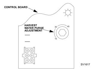
NOTE: The water purge **must be at the factory setting** of 45 seconds for the water inlet valve to energize during the last 15 seconds of the Water Purge. If set at 15 or 30 seconds the water inlet valve will not energize during the harvest water purge.
