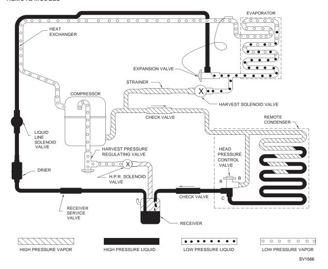
Figure 7-3. Remote Pre-Chill and Freeze Cycle (Models Q450/Q600/Q800/Q1000)
