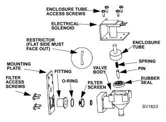
Figure 3-13. Exploded View of Water Inlet Valve
