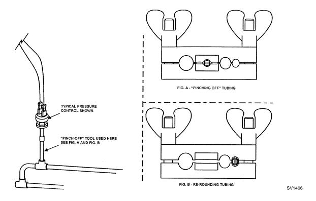
Figure 7-18. Using Pinch-Off Tool
