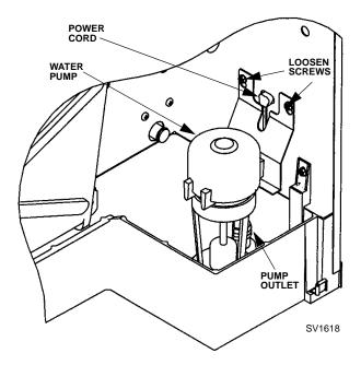
Figure 3-9. Water Pump Removal
