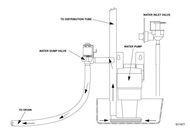
Figure 5-2. Water Flow Down the Drain
