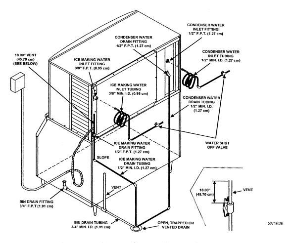
Figure 2-3. Typical Water Supply Drain Installation
