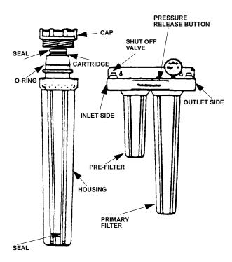
Figure 3-17. Typical Tri-Liminator® Water Filtration System
