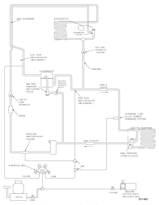
Figure 7-17. Remote Charging Connections
