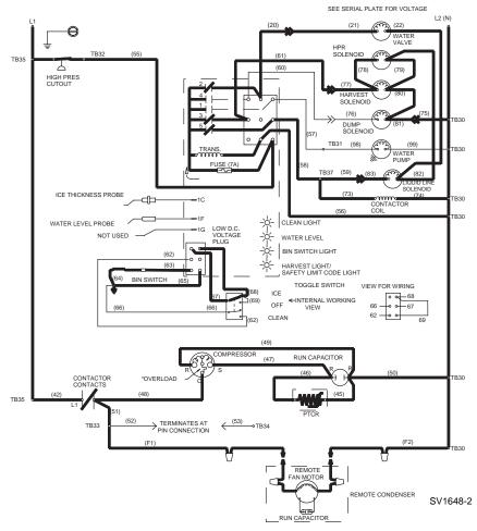
Figure 6-9. Remote — Refrigeration System Start-Up
