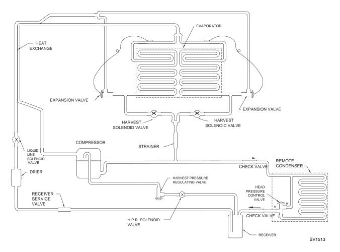
Figure 7-7. Q1300/Q1600/Q1800 Remote Models
