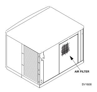
Figure 3-5. Self-Contained Air-Cooled Filter
