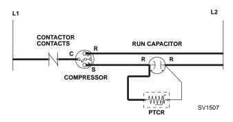
Figure 6-16. After Start-Up (Current Flows Through Run Capacitor)
