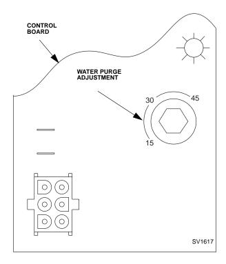
Figure 3-4. Water Purge Adjustment
