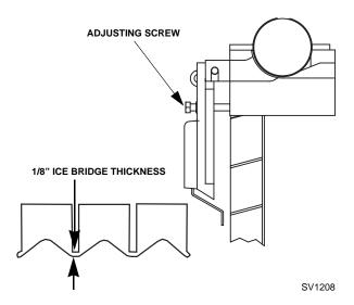
Figure 3-3. Ice Thickness Check
