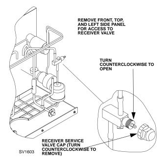
Figure 2-9. Backseating the Receiver Service Valve
