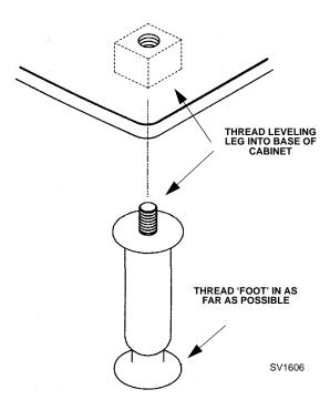
Figure 2-1. Leveling Leg and Foot
