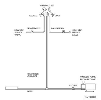
Figure 7-15. Charging Connections
