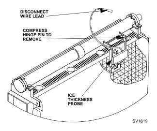
Figure 3-10. Ice Thickness Probe Removal
