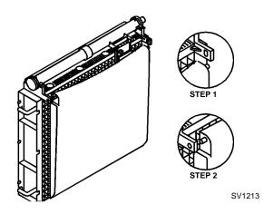
Figure 3-16. Water Curtain Removal
