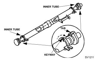
Figure 3-15. Water Distribution Tube Disassembly
