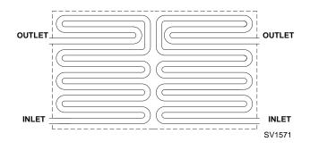
Figure 7-11. Q1300/Q1600/Q1800 Evaporator Tubing
