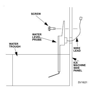
Figure 3-11. Water Level Probe Removal
