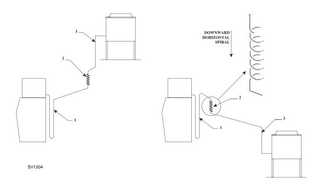
Figure 2-5. Routing Line Sets
