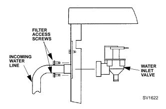
Figure 3-12. Water Inlet Valve Removal
