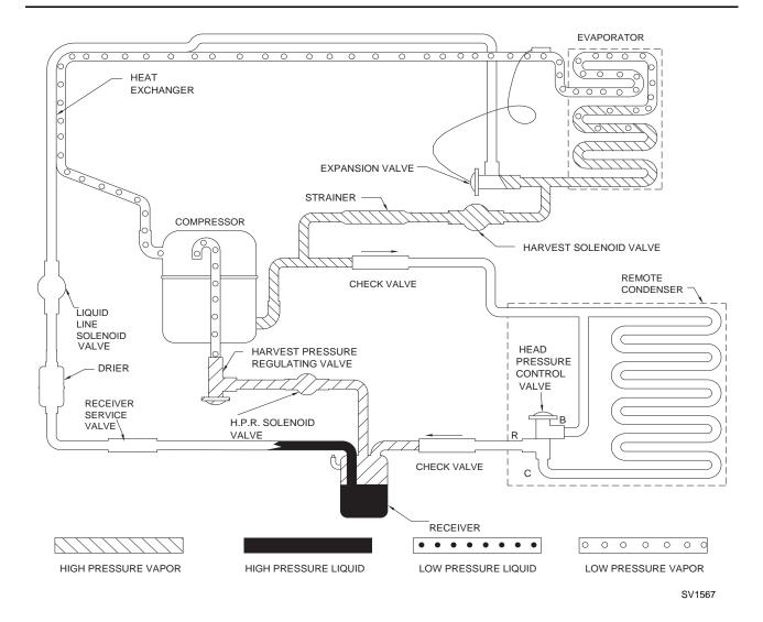
Figure 7-4. Remote Harvest Cycle (Models Q450/Q600/Q800/Q1000)
