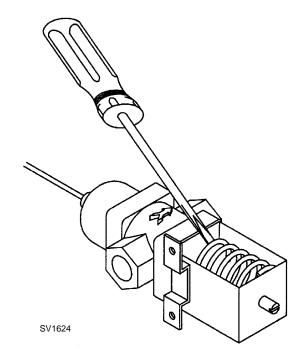
Figure 3-18. Pry Open the Water Regulating Valve
