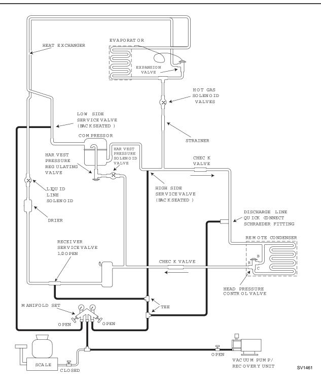
Figure 7-16. Recovery/Evacuation Connections
