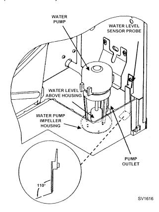
Figure 3-2. Water Level Probe
