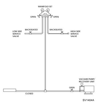
Figure 7-14. Recovery/Evacuation Connections
