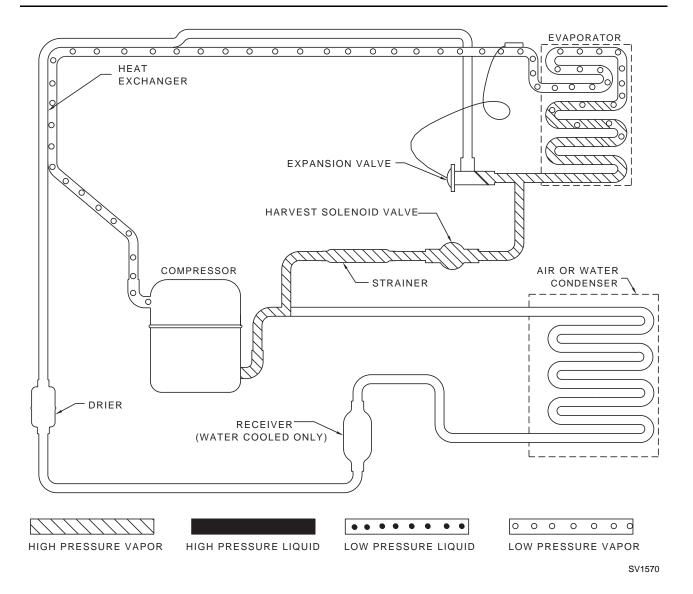
Figure 7-2. Self-Contained Harvest Cycle (Models Q200/Q280/Q320/Q370/Q420/Q450/Q600/Q800/Q1000) Harvest Cycle Refrigeration Sequence
