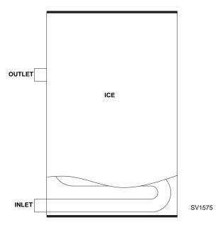
Figure 7-9. Extremely Thin Ice Formation at Evaporator Inlet
