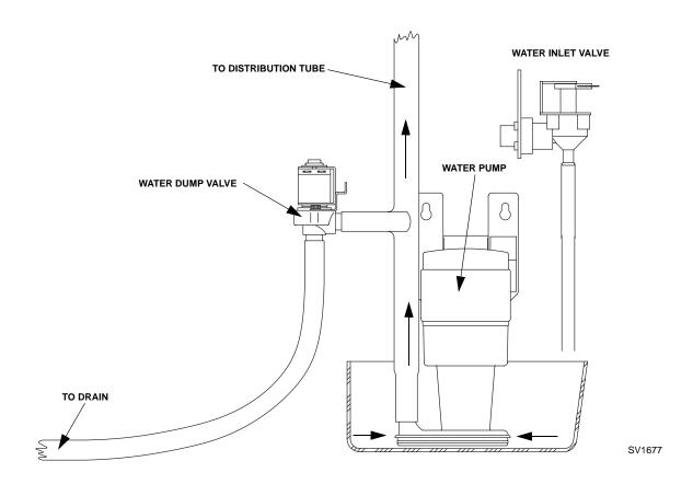
Figure 5-1. Water Flow Over the Evaporator
