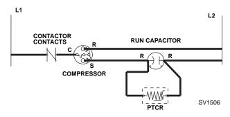
Figure 6-15. During Start-Up (First .25 - 1.0 Seconds)
