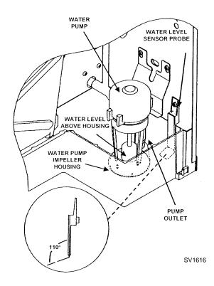
Figure 6-25. Freeze Cycle Water Level Setting
