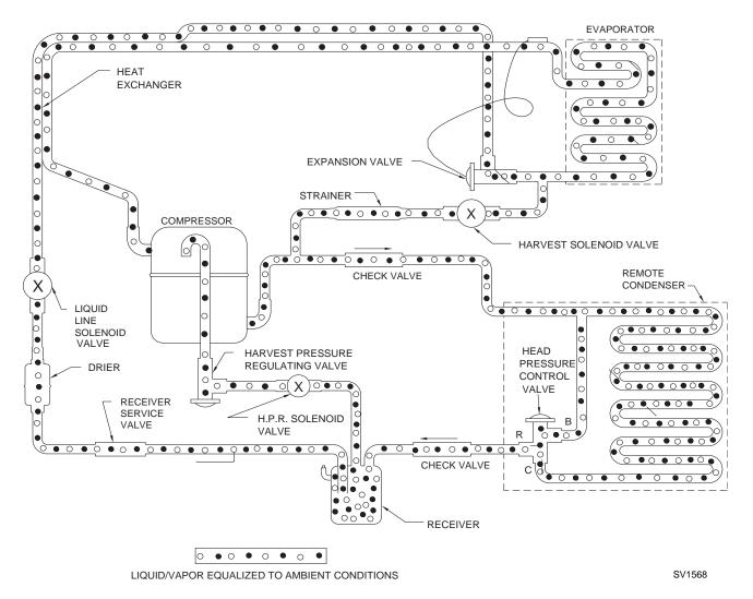
Figure 7-5. Remote Automatic Shut-Off (Models Q450/Q600/Q800/Q1000)
