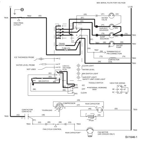
Figure 6-1. Self-Contained — Water Purge
