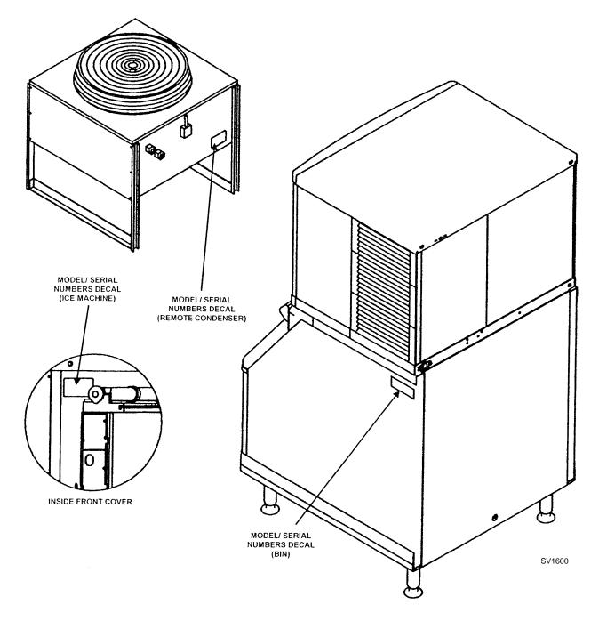
Figure 1-1. Model/Serial Number Location
