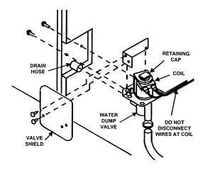
Figure 3-7. Dump Valve Removal
