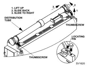
Figure 3-14. Water Distribution Tube Removal
