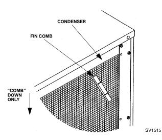
Figure 3-6. Straighten Bent Condenser Fins
