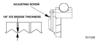
Figure 6-21. Ice Thickness Check
