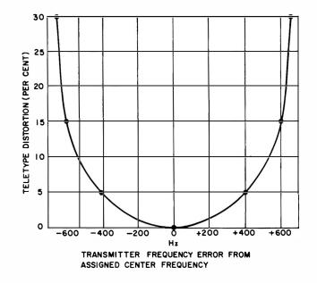
Figure 11-4. Single Channel FSK (±425 Hz) Transmission Test Data
