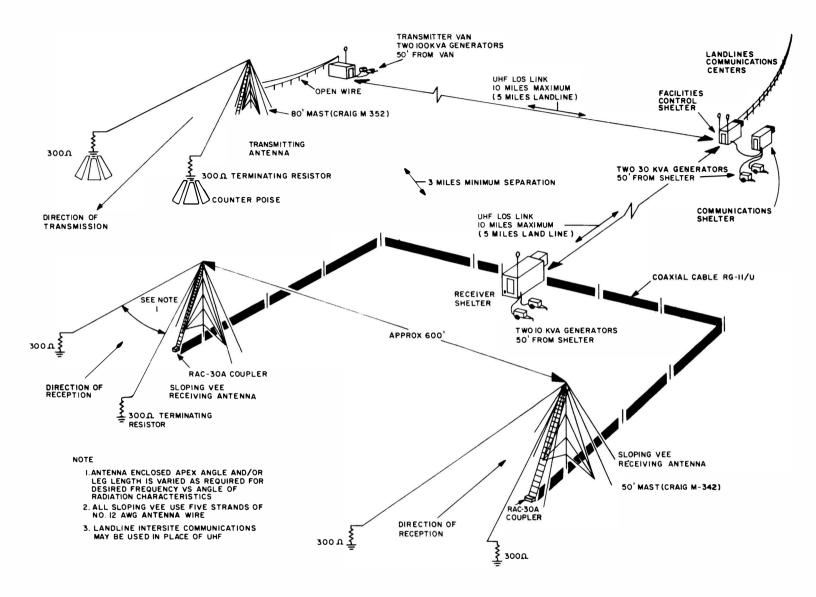
Figure 13-1. AN/TSC-18 System Facility and Antenna Plan
