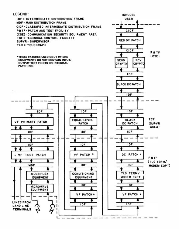
Figure 3-2. Typical Circuit Flow Through Communications Center Patching Facilities
