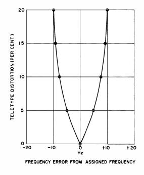
Figure 11-5. VFCT Channel Frequency Deviation Test Data
