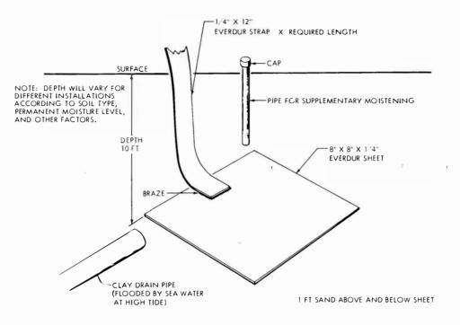
Figure 12-6. Everdur Ground Installation at USNRF, San Diego
