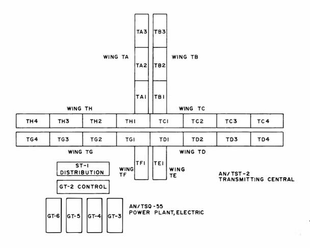
Figure 13-3. Site Plan, Transportable Transmitter Station
