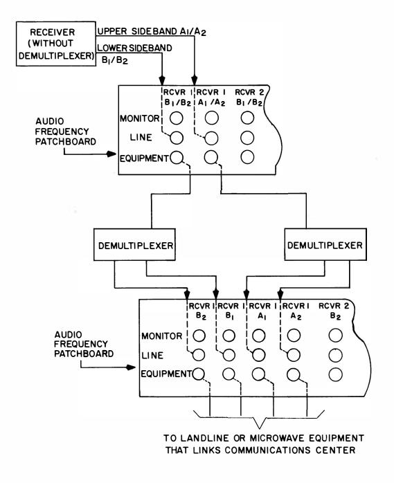
Figure 5-2. Receiver Patchboard (Separate Demultiplexer)
