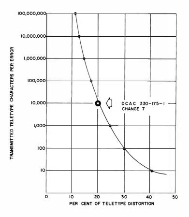
Figure 11-6. Teletype Distortion Rate Versus Error Rate
