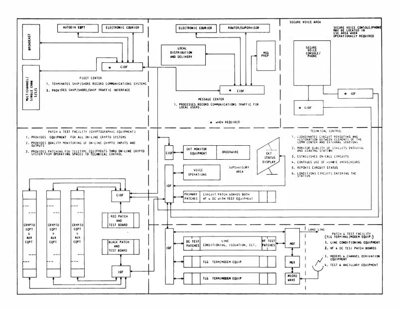
Figure 3-1. Functional Division Concept for Communication Center
