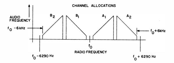
Figure 2-2. Independent Sideband Allocation
