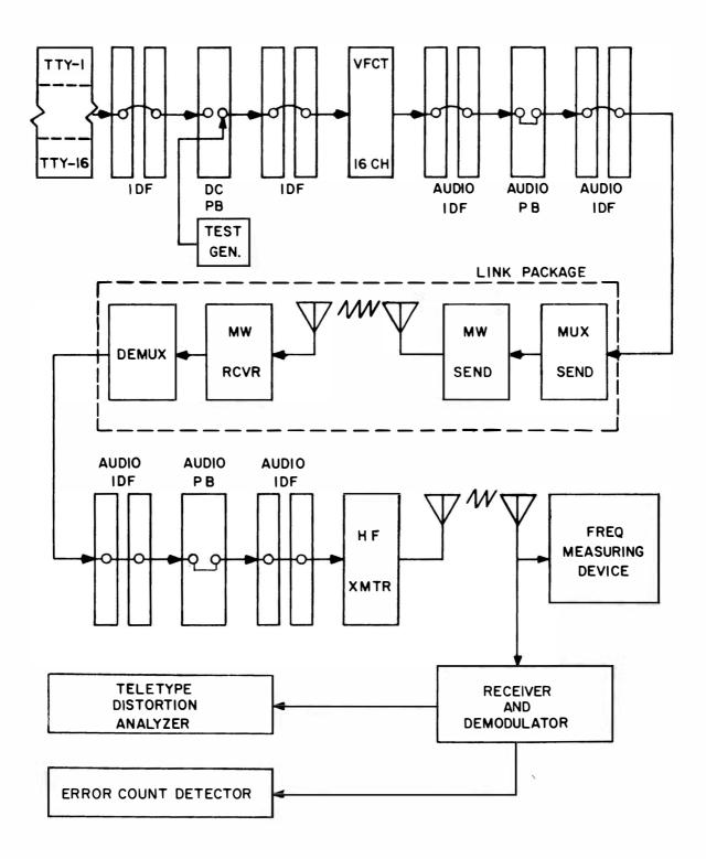
Figure 11-1. Typical Send Circuit Test
