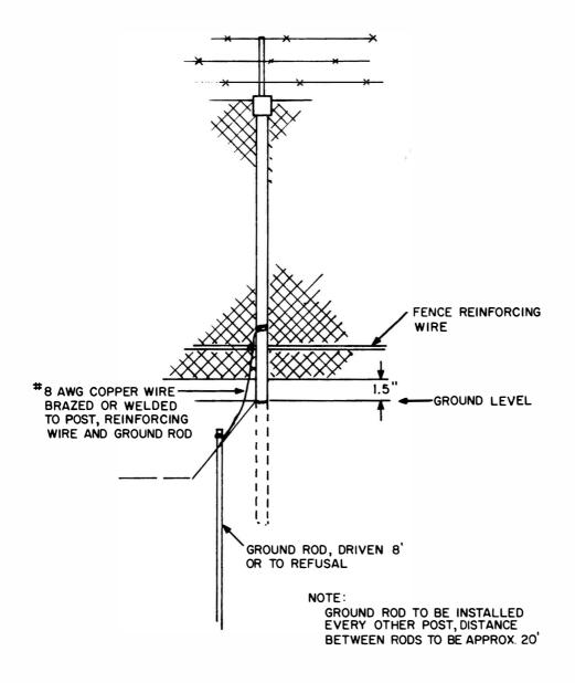
Figure 12-10. Typical Fence Grounding Plan
