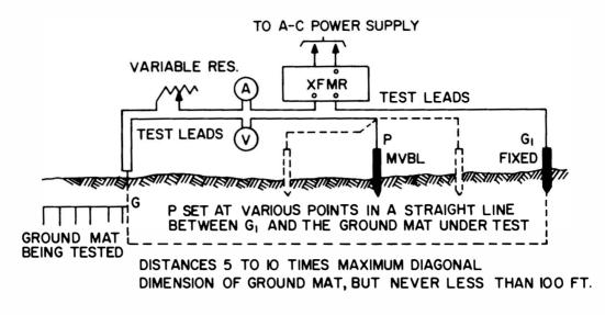
Figure 12-8. Fall-of-Potential Test Method
