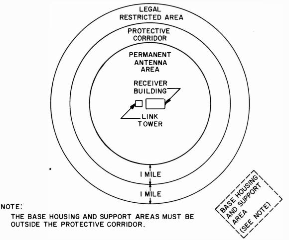
Figure 5-11. Receiver Station Site Plan
