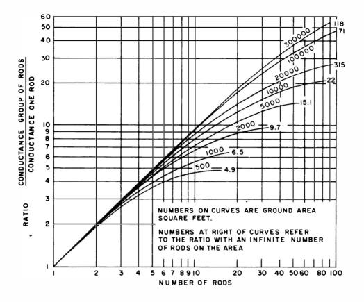
Figure 12-3. Conductance of Multiple Electrodes Versus Area
