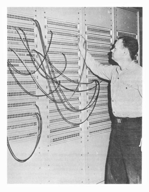
Figure 5-3. RF Receiver Coaxial Patchboard
