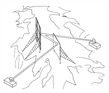
Figure 6-2. Passive Double Reflector
