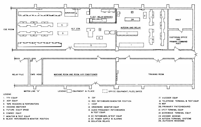
Figure 3-11. Typical Communications Center Layout (Sheet 3 of 3)
