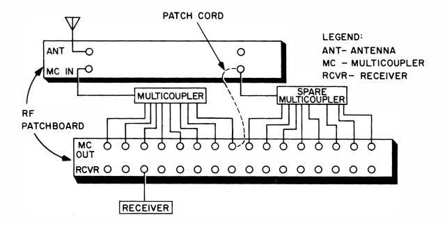
Figure 5-4. Multicoupler and Spare Multicoupler Installation
