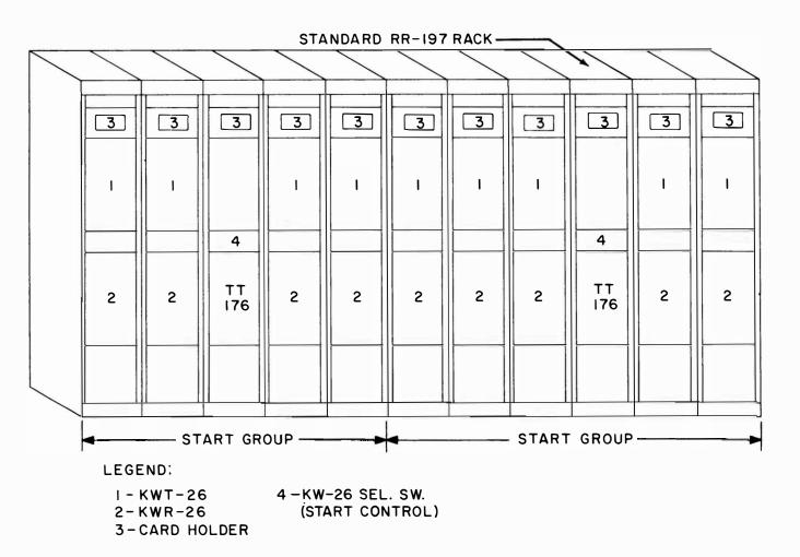
Figure 3-5. Typical Arrangement for Cryptographic and Restart Equipment
