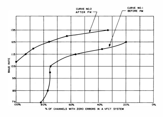
Figure 11-3. 3-kHz VFCT Receive System Test Results
