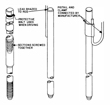
Figure 12-1. Grounding Rods
