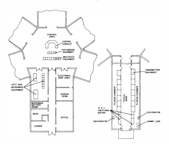
Figure 4-2. Large Transmitter Building and Plenum Concept
