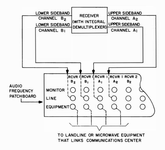
Figure 5-1. Receiver Patchboard (Integral Demultiplexer)
