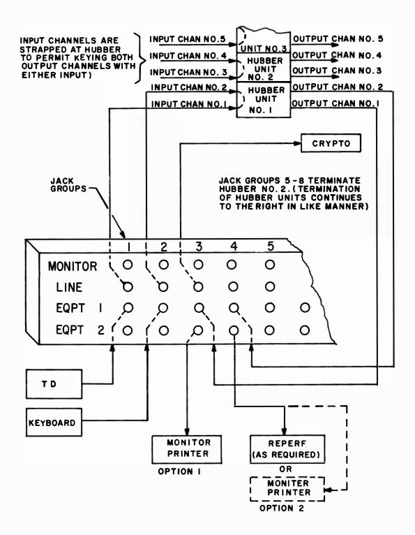
Figure 3-4. Hubber Unit Jack Field Arrangement
