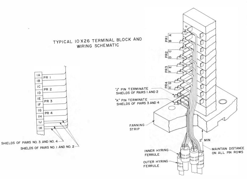
Figure 9-6. Intermediate Distribution Frame Terminal Blocks (Sheet 2 of 4) (Showing termination of individually shielded pair cables).
