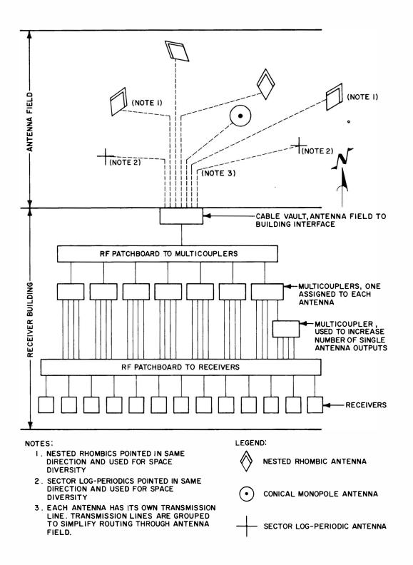
Figure 5-5. Normal Receiver Station Antenna RF Distribution
