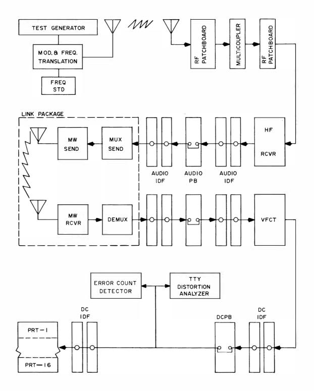
Figure 11-2. Typical Receive Circuit Test
