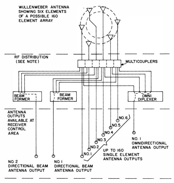
NOTE: EACH OF THE 160 ELEMENTS FEED THE RF DISTRIBUTION IN A SIMILAR MANNER, ADDITIONAL BEAM AND OMNIDIRECTIONAL UNITS ARE INSTALLED IN ACCORDANCE WITH OPERATIONAL REQUIREMENTS.
