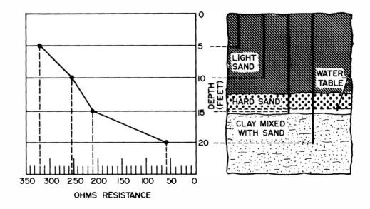
Figure 12-9. Electrode Depth Resistance
