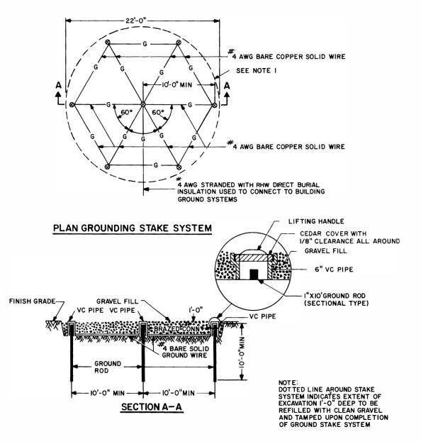
Figure 12-4. Multiple Driven Electrode Ground Plan
