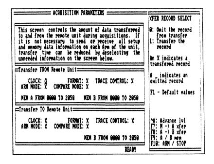
Figure 3-9. Acquisition Parameters Screen
