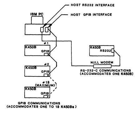
Figure 1-1. PC Equipment Connections
