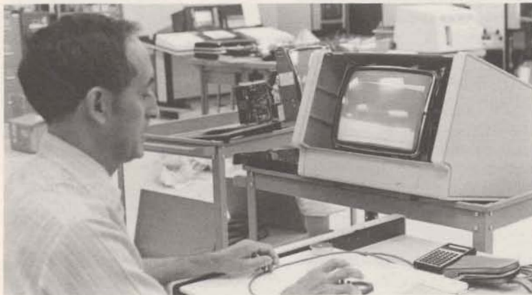
Will Florence tests a Genigraphics drawing tablet in the manufacturing department at Electronics Park in Syracuse. All Genigraphics equipment, from the smallest component to finished unit, is tested until the picture is perfect.
