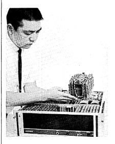
An engineer demonstrates how the core stack can be removed easily from the Model RGX core memory.
