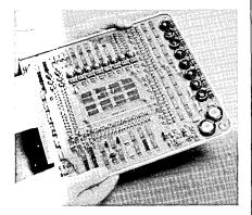
The MEMCARD system features cycle times of 1.5 microseconds. It is designed to operate in commercial environments of 0 to 50 degrees centigrade, and features temperature compensation within the memory itself, and plug-in convenience for easy maintenance or replacement. The 3-wire, 3D memory, contained on a plane in the center of the printed circuit card, is comprised of eight mats, each containing 1024 cores. (For more information, designate #48 on the Reader Service Card.)
