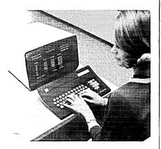
The System consists of a control unit, up to 12 operator display stations, and a rack of four tape recorders. A unique feature of the System 6000 is the automatic merging of data batches from all operators onto a single tape at very high speeds. In conventional systems, a special tape machine, or "pooler" is required to merge all the data on short "operator" tapes onto one reel prior to input into the computer.
