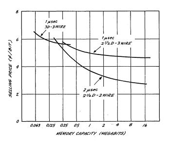
SYSTEMS INCLUDE ADDRESS REGISTERS , DECODERS , DRIVERS , SWITCHING, CORE STACKS , SENSE AMPLIFIERS , INPUT-DUTPUT REGISTERS , AND TIMING .
