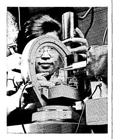
A U.S. Dept. of Agriculture laboratory technician positions a crystal for analysis on an X-ray diffractometer.
