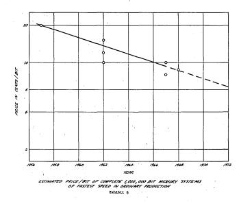
trend of core memories but have not substantially broken away from it. (The memories in the lower section of the chart are "scratch pad" memories, which are not directly comparable with main memories because they are not bound by the same economic constrictions.)
