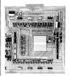
cuit card that will just fill a file holder. Cycle speed is 1 microsecond in the Read or Write mode and read data access time is 750 nanoseconds.
