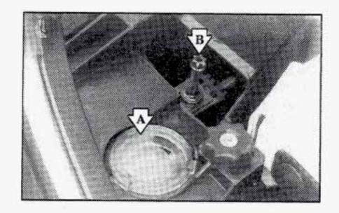
Check the vertical aim for each headlamp (A). The vehicle must be on a level surface. Turn the vertical aiming screw (B) until the bubble in the level is lined up with the 0 (zero).
