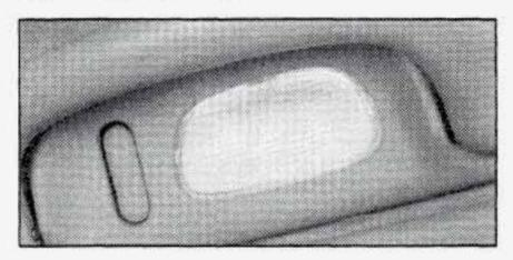
To turn on a rear seat reading lamp, press the switch above that rear door. To turn off the reading lamp, press the switch again.
