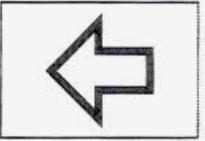
An arrow on the instrument panel will flash in the direction of the turn or lane change. If your vehicle is equipped with the Head-Up Display (HUD), an arrow will also appear in the display area to indicate the direction of the turn or lane change.
