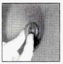
Unhook the cargo net from the cargo net retainer and remove the retainer by turning it to the left.
