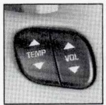
If your vehicle has this feature, you can control the temperature function by using the button on your steering wheel. Press the TEMP up arrow to increase the temperature and the TEMP down arrow to decrease the temperature.
