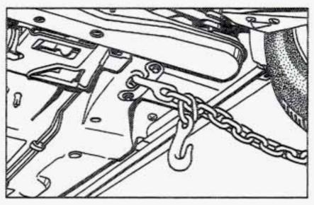
Attach T-hook chains on both sides in the slotted holes in the floor pan support rails just ahead of the rear wheels.
