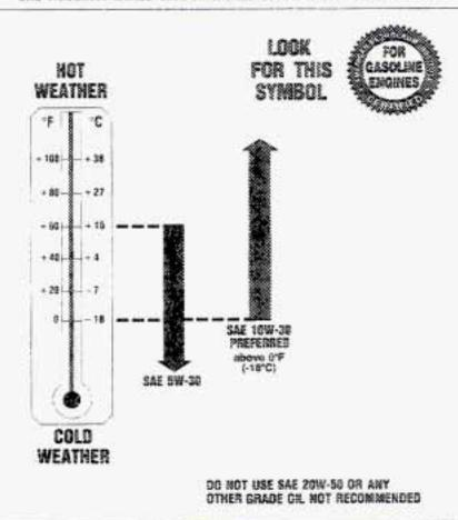
As shown in the chart, SAE 10W-30 is best for your vehicle. However, you can use SAE 5W-30 if it's going to be colder than 60°F (16°C) before your next oil change. When it's very cold, you should use SAE 5W-30. These numbers on an oil container show its viscosity, or thickness. Do not use other viscosity oils, such as SAE 20W-50.
