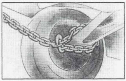
Attach a separate safety chain around the outboard end of each control arm.
