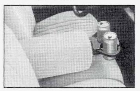
You may have a fold-down armrest between the front seats that opens into a storage area. To open it, pull up on the lever at the front edge. Inside are cupholders that can be rotated forward for use with the armrest cover closed. There is also a removable coinholder and a storage area for cassette tapes and compact discs.
