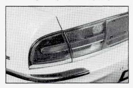
Turn lamps, stoplamps and back-up bulbs are located behind the taillamp assembly along the trunk lid. The following instructions explain how to access these bulbs.
