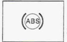
With the anti-lock brake system, the light(s) will come on when you start your engine and may stay on for several seconds. That's normal.
