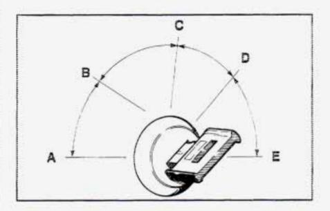
ACCESSORY (A): In this position you can operate your electrical power accessories. Press in the ignition switch as you turn the top of it toward you. LOCK (B): This is the only position from which you can remove the key. This position locks your ignition, steering wheel and transaxle. It's a theft-deterrent feature.
