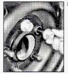
Install the compact spare tire on the wheel-mounting surface. Then replace the wheel nuts with the rounded end of the nuts toward the wheel. Tighten each nut by hand until the wheel is held against the hub.
