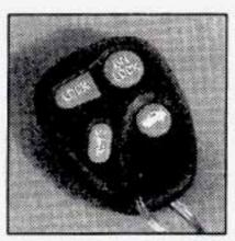
With the remote keyless entry system, you can lock and unlock your doors or unlock your trunk from about 3 feet (1 m) up to 30 feet (9 m) away using the remote keyless entry transmitter supplied with your vehicle. Your remote keyless entry system operates on a radio frequency subject to Federal Communications Commission (FCC) Rules and with Industry Canada.
