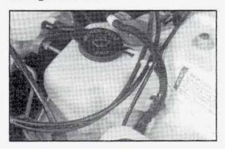
The windshield washer fluid reservoir is located by the coolant recovery tank on the driver's side of the engine compartment.
