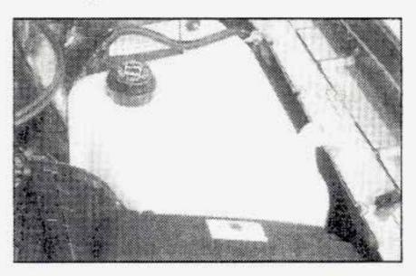
The coolant recovery tank is located on the driver's side of the engine compartment.
