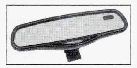
When set in the MIRROR position, this mirror automatically changes to reduce glare from headlamps behind you. A time delay feature prevents rapid changing from the day to night positions while driving under lights and through traffic. The mirror also includes an eight-point compass display in the upper right corner of the mirror face. When on, the compass automatically calibrates as the vehicle is driven.
