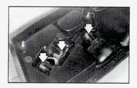
Pull the taillamp assembly away from the trunk lid. The bulbs are located on the back side of the assembly.
