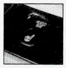
The heated seat controls are located next to the climate controls on the instrument panel. Press this button to turn on the heating element in the seat.
