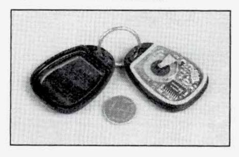
For battery replacement, use a Duracell® battery, type DL-2032, or a similar type.
