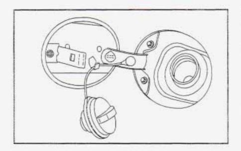
While refueling, hang the tethered cap on the fuel door latch.
