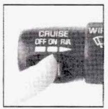
Once you're going about 25 mph (40 km/h) or more, you can move the cruise control switch from ON to R/A (Resume/Accelerate) for about half a second to reset. This returns you to your desired preset speed.
