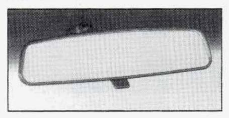
When you are sitting in a comfortable driving position, adjust the mirror so you can see clearly behind your vehicle. Grip the mirror in the center to move it up or down and side to side. The day/night adjustment allows you to adjust the mirror to avoid glare from the lamps behind you. Pull the tab forward for daytime use; push it back for night use.
