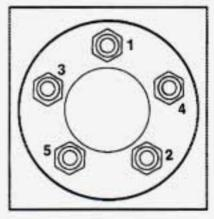
Using the wheel wrench, tighten the wheel nuts firmly in a crisscross sequence.
