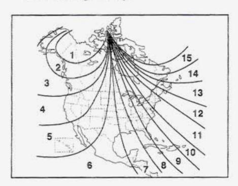
Press the COMPASS button on the bottom of the mirror until the new zone number appears in the display. After you stop pressing the button, the display will show a compass direction within a few seconds. (This is the automatic calibration mode. Drive in a circle to calibrate the mirror. See "Compass Calibration" following.)
