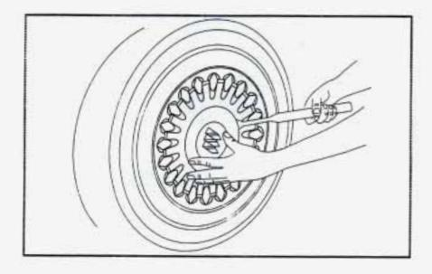
Insert the flat end of the wheel wrench in the notch and pry off the center cover. Do not drop the cover or lay it face down, as it could be scratched or damaged.
