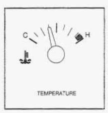
This gage measures the temperature of your engine. If the pointer moves into the red area, your engine is too hot. A temperature indicator light will turn on and a chime will sound.
