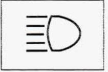
When the high beams are on, a light on the instrument panel will also be on. If your vehicle is equipped with HUD, this light will also appear in the display area.
