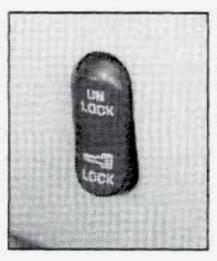
With power door locks, you can lock or unlock all doors of your vehicle by using either the driver or front passenger power door lock switch.
