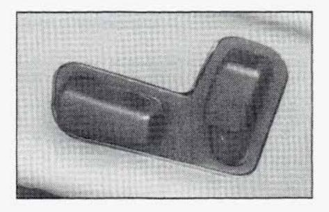
Raise or lower the front of the seat cushion by holding the front part of the horizontal control up or down.
