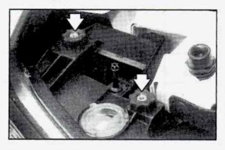
Each headlamp is attached by thumb screws.
