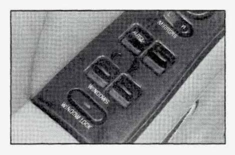
Switches on the driver's armrest control each of the windows while the ignition is on or retained accessory power is active. In addition, each passenger door has a switch for its own window.
