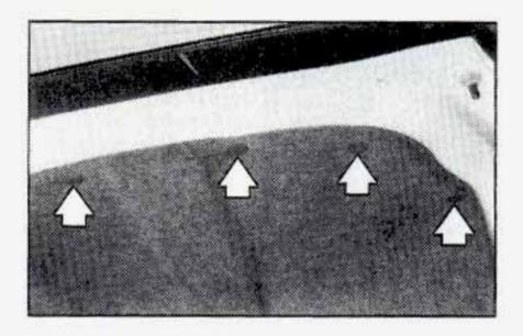
Next, there are eight fasteners along the top of the trunk lid (four on each side), holding the trunk trim in place. Remove these fasteners.
