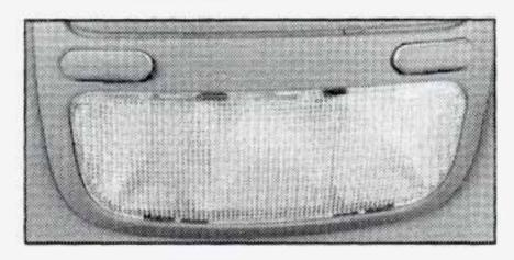
These lamps and the interior courtesy lamps will come on when you open a door. They will turn off when you turn on the ignition.
