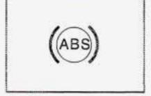
If there's a problem with the anti-lock brake system, this warning light will stay on. See "Anti-Lock Brake System Warning Light" in the Index.
