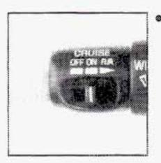
Push in the button at the end of the lever until you reach a desired lower speed then release it.
