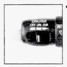
Use the accelerator pedal to go to a higher speed. Push the button at the end of the lever, then release the button and the accelerator pedal. You'll now cruise at the higher speed.
