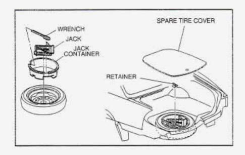
The compact spare tire is for temporary use only. Replace the compact spare tire with a full-size tire as soon as you can. See "Compact Spare Tire" later in this section.
