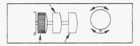
Pull the headlamp knob out to the first indent to turn on the parking lamps. Pull the knob out further, to the second indent to turn on the headlamps. Push the knob all the way back in to turn off the parking and headlamps.
