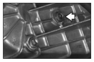
If the level is below the bottom of the filler plug hole, you'll need to add some lubricant. Add enough lubricant to raise the level to the bottom of the filler plug hole. Use care not to overtighten plug.
