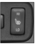
This control is located on the side of the seat. This feature will quickly heat the lower cushion and lower back of the driver and front passenger seats for added comfort.
