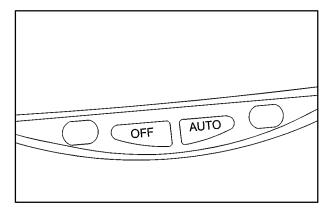
Press the AUTO button at the base of the mirror to turn on the automatic feature. The button has an indicator light to show it is on. Press the OFF button to turn the automatic feature off.
