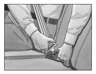
1. Pick up the latch plate and pull the belt across you. Don't let it get twisted. The shoulder belt may lock if you pull the belt across you very quickly. If this happens, let the belt go back slightly to unlock it. Then pull the belt across you more slowly. 2. Push the latch plate into the buckle until it clicks.
