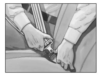
To unlatch the belt, just push the button on the buckle.
