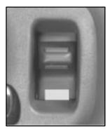
To unlock the door, slide the lever on your inside door up. You will see a red area on the lever.
