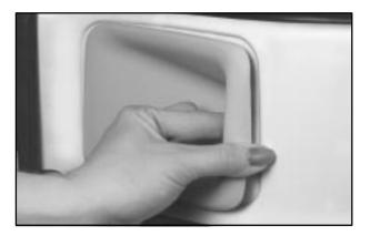
Before you can lower the spare tire, you must remove the access hole cover on the passenger's side of the rear bumper. Insert your index finger into the indentation near the lamp and pull to remove the cover.
