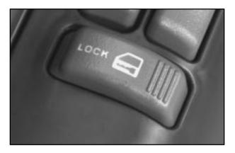
The power door lock switch is located on the armrest. Remove the ignition key and press LOCK to lock all the doors at once.
