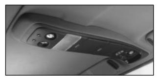
The overhead console includes reading lamps, a driver information system, a storage compartment for sunglasses and a HomeLink<sup>®</sup> transmitter.
