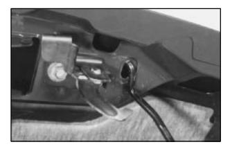
Lift the hood, release the hood prop from its retainer and put the hood prop into the slot in the hood. You may have a lamp that comes on when you lift the hood. When you lift the hood, you'll see these items:
