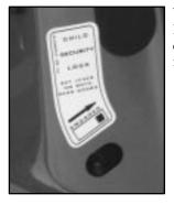
With this feature, you can lock the rear doors so they can't be opened from the inside by passengers.
