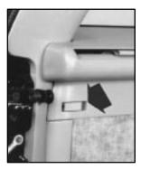
To remove your jack cover, pull up on the latches on the cover. Remove the wheel blocks, jack and wheel wrench.
