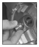
8. Put the nuts on by hand. Make sure the rounded end is toward the wheel. Tighten each nut by hand until the wheel is held against the hub. If a nut can't be turned by hand, use the wheel wrench and see your dealer as soon as possible.
