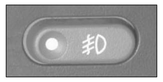
Use your fog lamps for better vision in foggy or misty conditions. Your low-beam headlamps or your parking lamps must be on for your fog lamps to work. The fog lamp switch is on the instrument panel under the lamps switch. Press the switch to turn the fog lamps on. Press the switch again to turn them off. A light will glow in the switch when the fog lamps are on.
