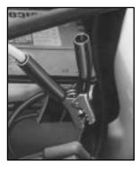
8. Now connect the black negative (-) cable to the good battery's negative (-) terminal. Don't let the other end touch anything until the next step. The other end of the negative cable doesn't go to the dead battery. It goes to a heavy unpainted metal part on the engine of the vehicle with the dead battery.
