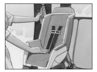
5. To tighten the belt, feed the shoulder belt back into the retractor while you push down on the child restraint. If you're using a forward-facing child restraint, you may find it helpful to use your knee to push down on the child restraint as you tighten the belt. 6. Push and pull the child restraint in different directions to be sure it is secure.
