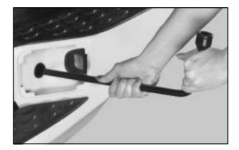
To remove the spare, insert the chisel end of the wheel wrench, on an angle, into the hole in the rear bumper. Be sure the chisel end of the wheel wrench connects into the hoist shaft.
