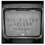
The access door for the remote oil filter is in the steering linkage shield assembly located under the radiator support. Twist the screw to unlock or lock the door. If you open the door, make sure it is securely closed when you are finished.
