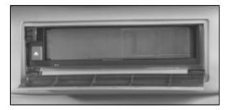
With the compact disc changer, you can play up to six discs continuously. Normal size discs may be played using the slots supplied in the magazine.
