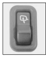
Your vehicle is equipped with power folding mirrors. This feature can be helpful when taking your vehicle through a car wash or through narrow spaces.
