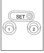
The memory seat control on the driver's seat looks like this. It is located on the left side of the driver's seat.
