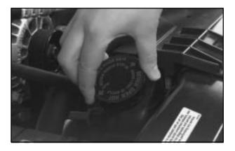
1. You can remove the radiator pressure cap when the cooling system, including the radiator pressure cap and upper radiator hose, is no longer hot. Turn the pressure cap slowly counterclockwise until it first stops. (Don't press down while turning the pressure cap.)
