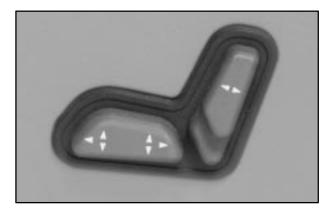
**Horizontal Control:** Raise the front of the seat by raising the forward edge of the button. Lower the front of the seat by lowering the forward edge of the button. Move the seat forward by moving the whole button toward the front of the vehicle.
