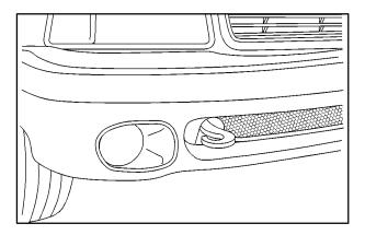
Your vehicle is equipped with recovery hooks. The recovery hooks are provided at the front of your vehicle. You may need to use them if you're stuck off-road and need to be pulled to some place where you can continue driving.
