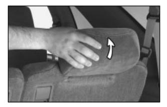
To return the head restraints to the upright position, reach behind the seats and pull the head restraint up until it locks into position.
