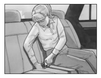
When you sit in the center rear seating position, you have a lap safety belt which has a retractor.
