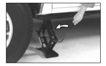
9. Lower the vehicle by turning the jack handle counterclockwise. Lower the jack completely.
