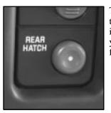
This button to the right of the steering wheel on the instrument panel allows you to release the liftglass from inside the vehicle.
