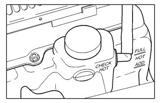
The vehicle must be on a level surface. When your engine is cold, the coolant level should be at ADD, or a little higher. When your engine is warm, the level should be up to FULL HOT, or a little higher.
