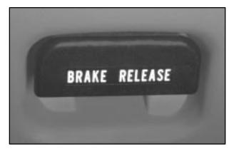
Pull the BRAKE RELEASE lever fully. It is located on the bottom of the driver's side of the instrument panel.
