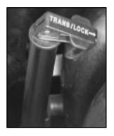
1. The transmission dipstick is located at the rear of the engine compartment.
