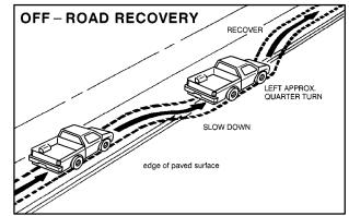
If the level of the shoulder is only slightly below the pavement, recovery should be fairly easy. Ease off the accelerator and then, if there is nothing in the way, steer so that your vehicle straddles the edge of the pavement. You can turn the steering wheel up to one-quarter turn until the right front tire contacts the pavement edge. Then turn your steering wheel to go straight down the roadway.
