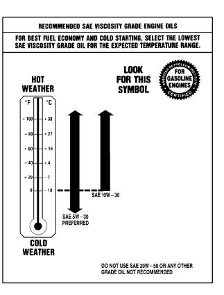
As shown in the chart, SAE 5W-30 is best for your vehicle. However, you can use SAE 10W-30 if it's going to be  $0^{\circ}F$  (-18°C) or above. These numbers on an oil container show its viscosity, or thickness. Do not use other viscosity oils, such as SAE 20W-50.
