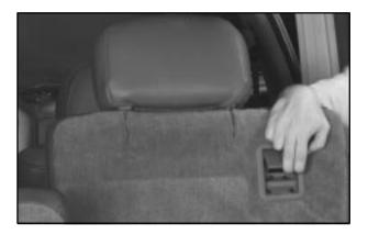
The rear seat release handles are on the rear of the seatbacks. Push back on the seatbacks as you pull up on the handles. The head restraint will automatically fold out of the way when the seatback is folded down.
