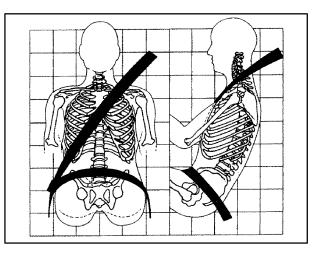
The lap part of the belt should be worn low and snug on the hips, just touching the thighs. In a crash, this applies force to the strong pelvic bones. And you'd be less likely to slide under the lap belt. If you slid under it, the belt would apply force at your abdomen. This could cause serious or even fatal injuries. The shoulder belt should go over the shoulder and across the chest. These parts of the body are best able to take belt restraining forces.
