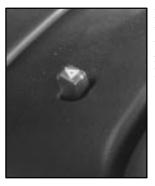
Press the button on top of the steering column all the way down to make your front and rear turn signal lamps flash on and off.
