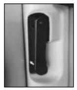
To open the hood, first pull the handle inside the vehicle on the lower driver's side of the instrument panel. Then go to the front of the vehicle and release the secondary hood release.
