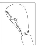
Your vehicle is equipped with a tow/haul selector switch. This switch is located on the shift knob.
