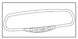
This mirror automatically changes to reduce glare from headlamps behind you. A photocell on the back of the mirror senses when it is becoming dark outside. Another photocell built into the mirror surface senses when headlamps are behind you.
