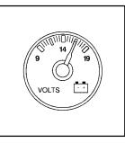
When your engine is not running, but the ignition is on (in RUN), this gage shows your battery's state of charge in DC volts.
