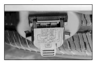
Your vehicle is equipped with the seven-wire trailer towing harness. This harness has a seven-pin universal heavy-duty trailer connector that is attached to a bracket on the hitch platform. The seven-wire harness contains the following trailer circuits:
