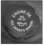
The engine oil fill cap is located in the engine compartment toward the passenger's side of the vehicle. See "Engine Compartment Overview" in the Index for more information on location.
