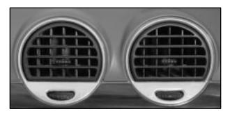
Your vehicle has air outlets that allow you to adjust the direction and amount of airflow inside the vehicle. Move the outlet up or down and move the control in the center of each outlet side-to-side to direct the air from the outlet. Use the thumbwheel under the outlet to turn the outlet off. For the most efficient airflow and temperature control, keep the outlet in the fully opened position.
