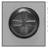
The driver's and passenger's seatback lumbar support can be adjusted four ways by moving a single control located on the outboard side of the seat cushions.
