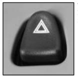
The button for the hazard warning flashers is located on top of the steering column.
