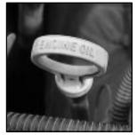
The engine oil dipstick handle is a yellow ring located in the engine compartment toward the passenger's side of the vehicle. See "Engine Compartment Overview" in the Index for more information on location.
