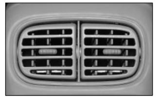
The rear seat outlets can be used to adjust the airflow toward either seating area, the floor or upward. Move the control in the center of each outlet in any direction to direct airflow.
