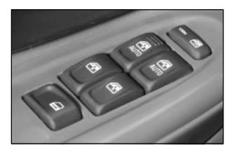
The controls for the power windows are located on the armrest on each of the side doors. With power windows, the switches operate the windows when the ignition is in RUN, ACCESSORY or when Retained Accessory Power (RAP) is active. (See "Retained Accessory Power" in the Index.) The driver's door has a switch for each of the passenger's windows as well.
