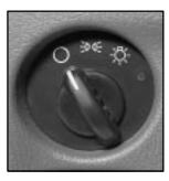
Your exterior lamps knob is located on the driver's side of your instrument panel.
