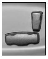
The power seat controls are located on the outboard side of the front seat cushions.
