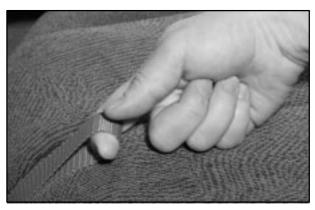
Pull up on the tab located where the seat cushion meets the seatback to fold the seat cushion up and out of the way. This will allow the seatback to fold flat and increase the cargo area.
