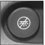
You can use the dome override button, located below the exterior lamps knob, to set the dome lamps to come on automatically when a door is opened, or to remain off.
