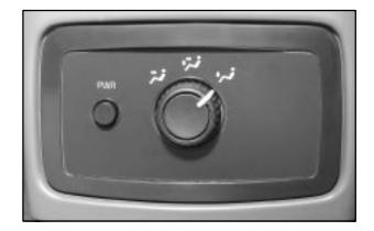
The temperature of the air coming through the rear outlets is determined by the front passenger's temperature setting. Press the PWR button to turn the rear comfort controls on and off. Use the mode knob to change the direction of airflow (upper, bi-level or floor) to the rear seat area.
