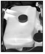
The engine coolant r ecovery tank is in the engine compartment on the passenger's side of the vehicle. See "Engine Compartment Overview" in the Index for more information on location.
