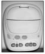
The overhead console includes sunglasses storage, a HomeLink® transmitter and a travel note recorder (if equipped).
