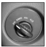
If your vehicle is equipped with the automatic transfer case, the transfer case knob is located to the right of the steering wheel on the instrument panel. Use this knob to shift into and out of four-wheel drive.
