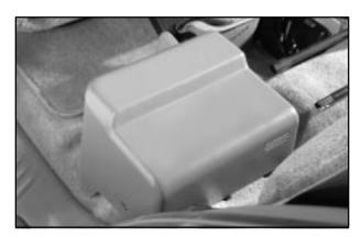
The rear underseat fuse block is located under the rear seat on the driver's side of the vehicle.
