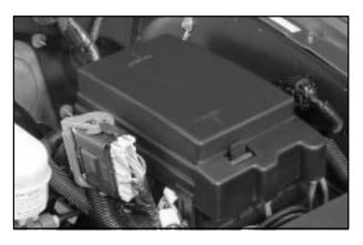
The fuse block is located under the hood in the engine compartment on the driver's side of the vehicle. See "Engine Compartment Overview" in the Index for more information on location.
