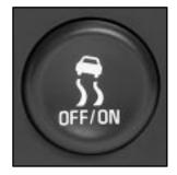
To turn the system on or off press the TAS on/off button located near the shift lever. If you used the button to turn the system off, the TRAC OFF light on the button will come on and stay on.
