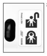
2. You will find a security lock lever located on the inside edge of each rear door. Move the lever down to engage the safety lock. Move the lever up to disengage the safety lock.
