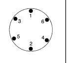
12. Use the wrench to tighten the wheel nuts firmly in a crisscross sequence as shown.
