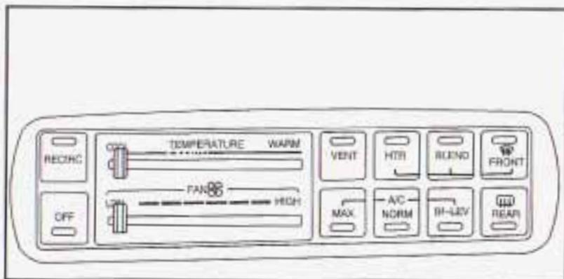
**TEMPERATURE:** This lever is used to adjust the temperature of the air coming through the system. Moving the lever between COOL and WARM will change the temperature of the air coming through your outlets.
