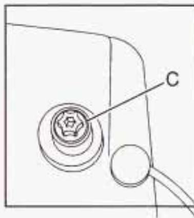
5. Turn the vertical aiming screw (C) until the headlamp beam is aimed to the horizontal tape line.
