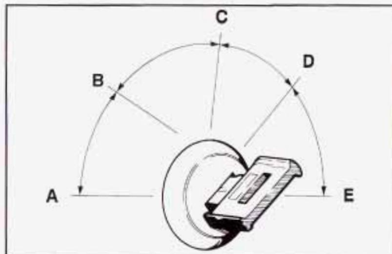
**(A) ACCESSORY:** This position lets you use your electrical accessories such as power windows, power sunroof (if equipped), radio and the windshield wipers. To use, push in the ignition key and turn it toward you. Your steering wheel will remain locked, just as it was before you inserted the key.
