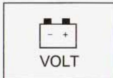
When you turn the key to RUN, this light will turn on briefly to show that the generator and battery charging systems are working.
