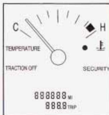
This gage shows the engine coolant temperature. If the pointer moves into the shaded area, the engine is too hot.
