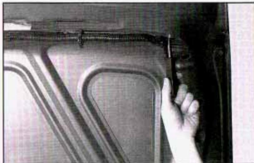
1. Open the trunk. Loosen and remove the seven fasteners that hold the taillamp assembly in place. The assembly for both sides is one piece. The entire piece must be removed to replace any bulbs.
