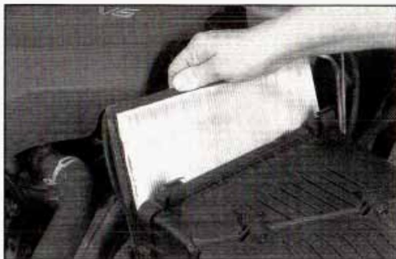
Refer to *Part A: Scheduled Maintenance Services* on page 6-4 to determine when to replace the air filter.
