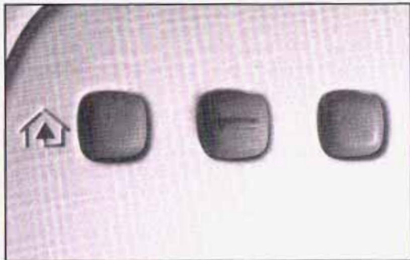
HomeLink<sup>®</sup>, a combined universal transmitter and receiver, provides a way to replace up to three hand-held transmitters used to activate devices such as gate operators, garage door openers, entry door locks, security systems and home lighting. Additional HomeLink<sup>®</sup> information can be found on the internet at [www.homelink.com](http://www.homelink.com) or by calling 1-800-355-3515.
