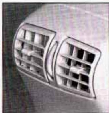
In vehicles equipped with rear seat outlets, you can adjust the direction of the airflow using the lever in the center of each outlet. Use the thumbwheel located between the outlets to turn them on and off.
