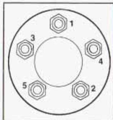
11. Tighten the wheel nuts firmly in a crisscross sequence.
