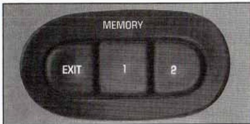
If your vehicle has this feature, the controls are located on the driver's door panel, and are used to program and recall memory settings for the driver's seating, outside mirror positions and climate controls. See *Climate Control System on page 3-23* for more information.
