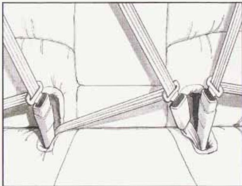
1. Buckle the center passenger position safety belt, then route the safety belts through the proper slots in the seat cushion. Don't let the safety belts get twisted.
