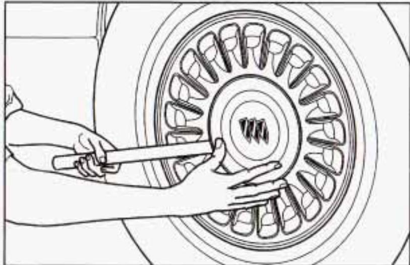
If your vehicle has an aluminum wheel with a center cover that hides the wheel nuts, remove the center cover by using the flat end of the wheel wrench to pry it off.
