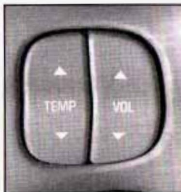
If your vehicle has this feature, you can control the temperature function by using the switch located on your steering wheel.
