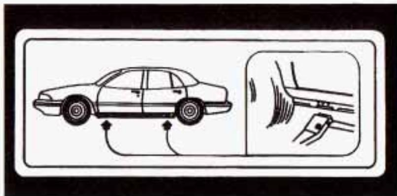
4. Put the jack into a notch in the frame which is located near each wheel well. The front notch is eight inches (20 cm) back from the front wheel well. The rear notch is three inches (8 cm) forward from the rear wheel well. The notches are accessible through openings in the plastic trim at the bottom of the vehicle.
