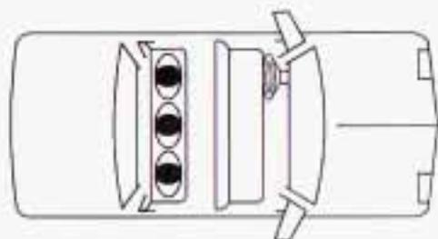
Your vehicle has the LATCH system. You'll find anchors (A) in all three rear seat positions.
