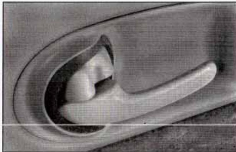
To unlock the door from the inside, move the manual door lock, located above the door handle, rearward. To lock the door, move the manual door lock forward.
