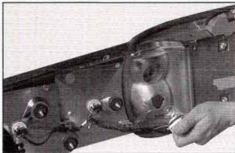
3. Push in the tab and turn the bulb socket counterclockwise to remove it.
