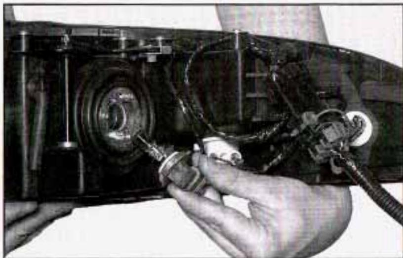
4. Turn the bulb retainer counterclockwise to remove it from the bulb assembly.
