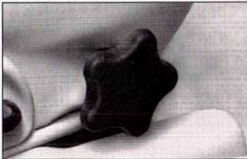
The knob that controls this feature is located on the outboard side of each front seat. Turn the knob toward the front of the vehicle to increase lumbar support. Turn the knob toward the rear of the vehicle to decrease lumbar support.
