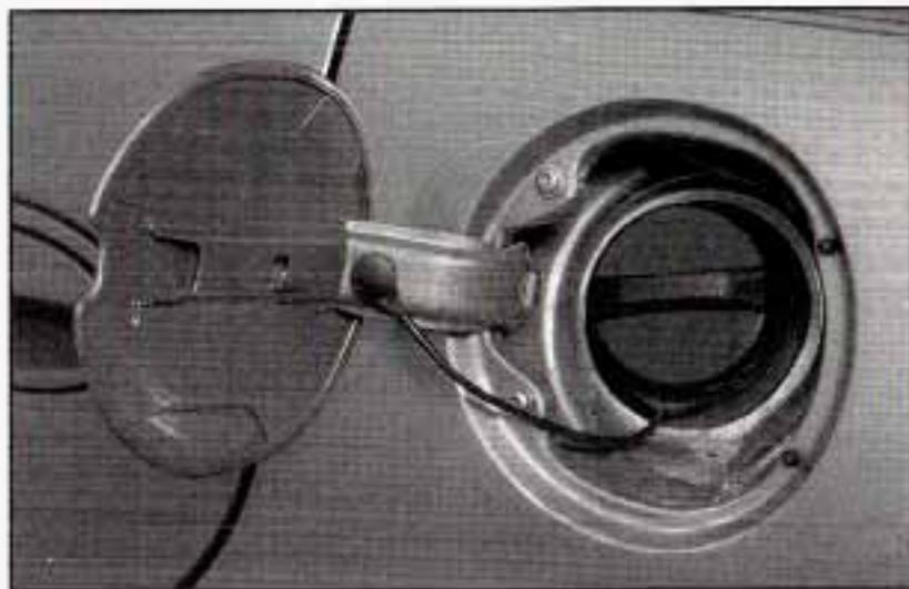
The fuel cap is behind a hinged fuel door on the driver's side of the vehicle.
