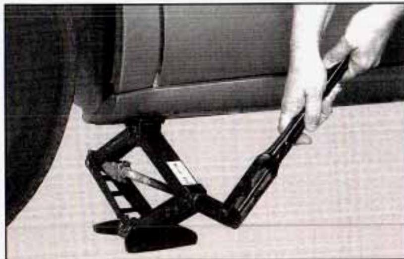
5. Raise the vehicle by turning the wheel wrench clockwise in the jack. Raise the vehicle far enough so there's enough room for the spare tire to fit under the wheel well.
