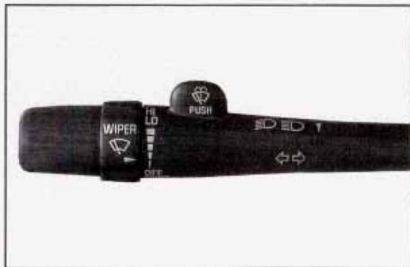
The windshield wipers are controlled by turning the band marked WIPER.
