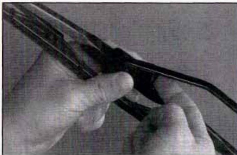
2. Push the tab on the wiper blade assembly and pull the assembly down enough to release it from the "U" hooked end of the wiper arm. Slide the assembly away from the arm.
