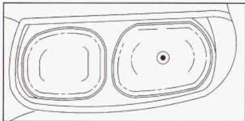
2. Measure the distance from the ground to the aim dot on each lamp; if left low beam, subtract two inches. Record this distance.
