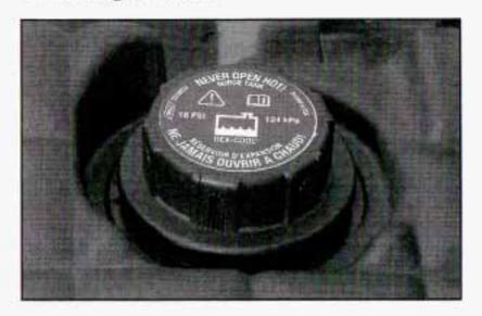
The engine coolant surge tank is located in the engine compartment on the driver's side of the vehicle. See Engine Compartment Overview on page 5-14 for more information on location.
