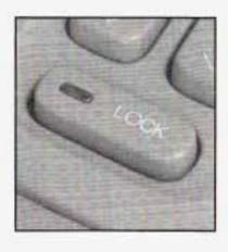
The rear window lockout button is located on the driver's door armrest next to the window switches.
