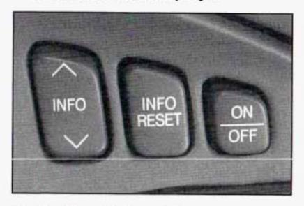
The Driver Information Center (DIC) buttons are located to the right of the steering wheel on the instrument panel, near the air outlets. ∧ INFO ∨ (Information): Pressing this button up or down will display the OUTSIDE TEMP, MILES RANGE, MPG AVG, MPG INST, GAL FUEL USED, AVG MPH, TIMER, BATTERY VOLTS, LF-RF-LR-RR TIRE (If Equipped), ENGINE OIL LIFE, TRANS FLUID LIFE, PHONE (Option) and FEATURE PROGRAMMING and Blank Display.
