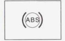
With the anti-lock brake system, the light(s) will come on when your engine is started and may stay on for several seconds. That's normal.
