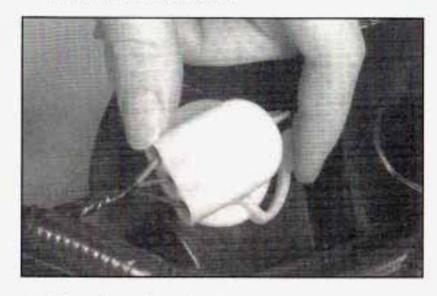
Press the bulb socket tab and turn the bulb socket counterclockwise to unlock the socket from the lamp housing.
