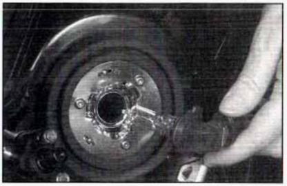
7. Remove the headlamp bulb socket.
