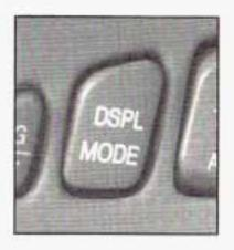
This button is located between the RESET TRIP A/B button and the ENG/MET button to the left of the steering wheel on the instrument panel.
