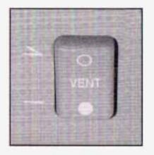
The two switches that operate the optional sunroof are located on the overhead console and include VENT, ROOF, open and close.
