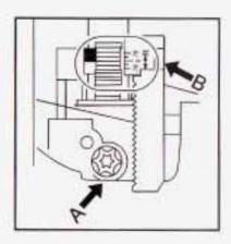
Turn the horizontal aiming screw (A) until the indicator (B) is lined up with zero.
