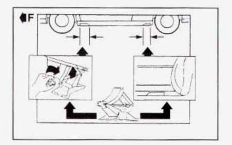
Find the jacking location from the diagram above and corresponding hoisting notches located in the plastic molding. The front location is 9.0 inches (23 cm) from the rear edge of the front wheel well, and the rear location is 2.5 inches (7 cm) from the front edge of the rear wheel well.
