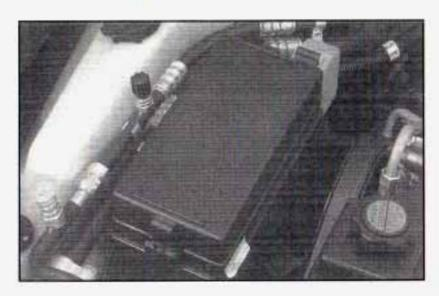
The underhood fuse block is located in the front of the engine compartment between the windshield washer fluid reservoir and the power steering fluid reservoir on the passenger's side of the vehicle. See Engine Compartment Overview on page 5-14 for more information on location.
