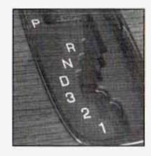
Move the shift lever into PARK (P) by pushing the lever all the way toward the front of your vehicle and then to the left.
