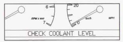
If the CHECK COOLANT LEVEL message comes on and stays on, it means you're low on engine coolant.
