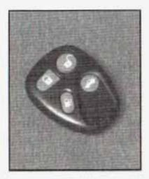
Lock): Press this button to lock the doors. The parking lamps will flash once and the horn will sound once. Pressing lock arms the theft-deterrent system.
