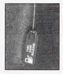
An alternate fuel door release strap is located inside the trunk on the driver's side of the vehicle.
