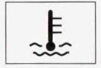
This light tells you that your engine has overheated. As a check, the light should come on for a few seconds when you start your engine.
