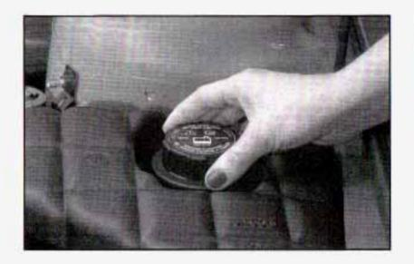
Park the vehicle on a level surface. You can remove the coolant surge tank pressure cap when the cooling system, including the coolant surge tank pressure cap and upper radiator hose, is no longer hot. Turn the pressure cap slowly counterclockwise (left) about one-quarter turn and then stop.
