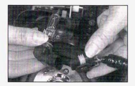
After removing the wiring harness connector from the headlamp bulb socket, replace the bulb assembly. Reconnect it to the wiring harness and reinstall the headlamp bulb assembly back into the headlamp housing.
