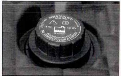
Then replace the pressure cap. Be sure the pressure cap is hand-tight and fully seated.
