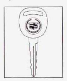
When trying to start the vehicle, if the engine does not start and the SECURITY light comes on, the key may have a damaged transponder. Turn the ignition off and try again.
