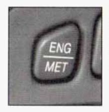
By pressing this button located to the left of the steering wheel on the instrument panel, you can go back and forth from English (miles) to metric (kilometers).
