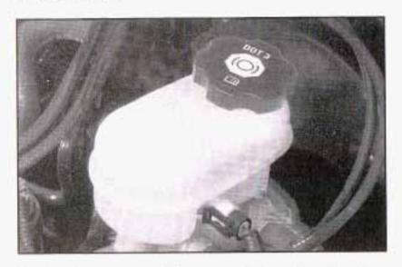
Your brake master cylinder reservoir is on the driver's side of the engine compartment. It is filled with DOT-3 brake fluid. See Engine Compartment Overview on page 5-14.
