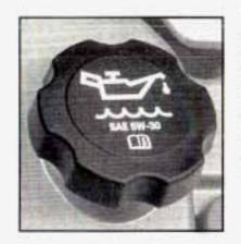
The engine oil fill cap is located behind the radiator on the passenger's side of the vehicle. For more information on location, see Engine Compartment Overview on page 5-14.
