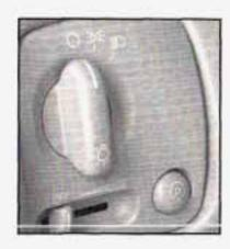
The control located on the left side of the instrument panel operates the exterior lamps.
