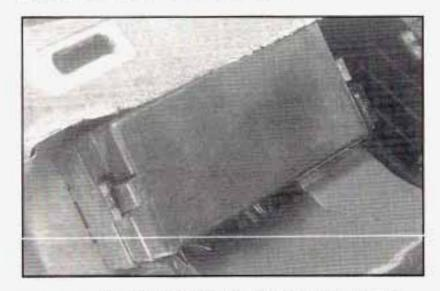
This fuse block is located under the rear seat on the driver's side of the vehicle. The rear seat cushion must be removed to access the fuse block. See *Removing* the Rear Seat Cushion listed previously in this section.
