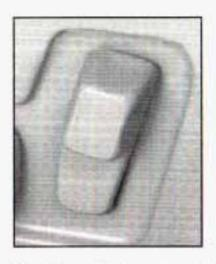
The switches used to adjust the front head restraints are located on the outboard side of each front seat.
