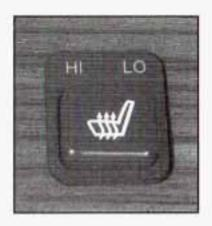
The front seat controls are located in the center console. The rear seat controls are located on the rear doors.
