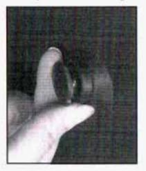
Remove the rear compartment sill plate by removing the upper convenience net retainers, located at each end, as shown.
