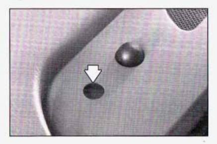
The light sensor for the Daytime Running Lamps (DRL) and the Twilight Sentinel® is located on the driver's side of the front defogger grille.
