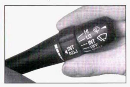
You can control the windshield wipers by moving the lever with the wiper symbol on it. This lever is located on the right side of your steering column. For information on wiper-activated headlamp operation, refer to Exterior Lamps on page 3-15.
