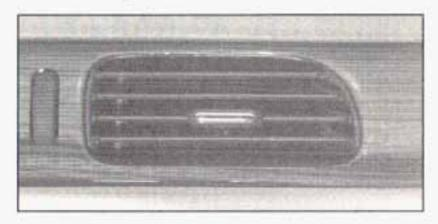
Use the levers located in the center of each outlet to change the direction of the airflow. Use the thumbwheels to open or close the outlets.
