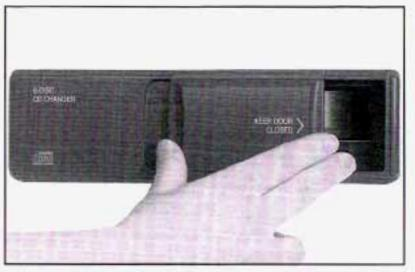
Close the door by sliding it all the way to the right. When the door is closed, the changer will begin checking for discs in the magazine. This will continue for up to one and a half minutes, depending on the number of discs loaded.
