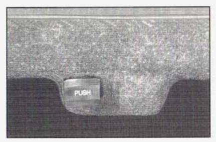
Your vehicle may be equipped with a rear seat pass-through door. The button for this feature is located in the trunk.
