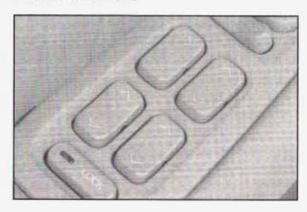
The power window switches are located on the armrest near each window. Press the up or down arrows on the switches to raise or lower the windows. Your vehicle has Retained Accessory Power (RAP) that allows you to use the power windows once the ignition has been turned off. For more information, see Retained Accessory Power (RAP) under Ignition Positions on page 2-22.
