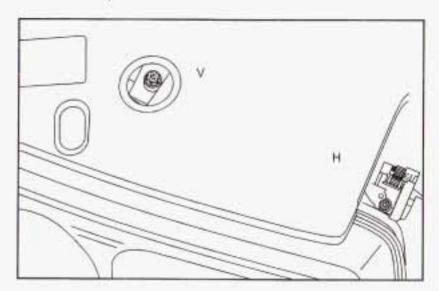
If you believe your headlamps need horizontal (left/right) adjustment, follow the horizontal aiming procedure. If you believe your headlamps need only vertical (up/down) adjustment, follow only the vertical aiming procedure.
