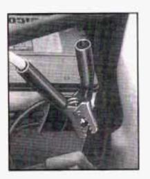
Now connect the black negative (-) cable to the negative (-) terminal location of the vehicle with the good battery. Use a remote negative (-) terminal if the vehicle has one. Don't let the other end of the cable touch anything until the next step. The other end of the negative (-) cable doesn't go to the dead battery. It goes to a heavy, unpainted metal engine part or to a remote negative (-) terminal on the vehicle with the dead battery.
