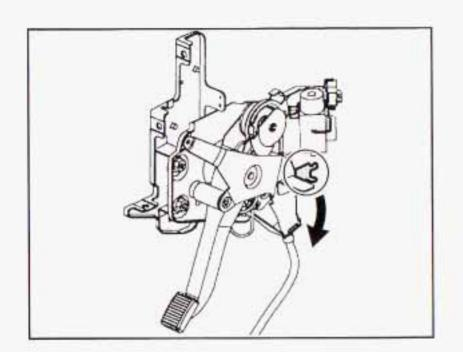
Reach under the driver's side of the instrument panel and pull down on the manual release lever, which is located behind the parking brake pedal. Pull down on the yellow tab as shown by the arrow in the illustration. If the parking brake does not release, you should have your vehicle towed to your dealer for service.
