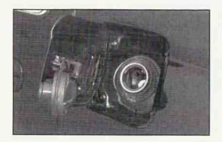
While refueling, hang the fuel cap by the tether from the hook on the fuel door.
