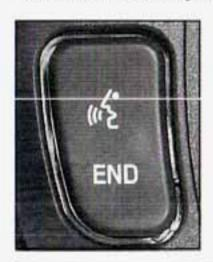
The controls are located on the left side of the steering wheel. Press the top part of the control to access OnStar<sup>®</sup>. You will hear a ready prompt from the system, and then you can begin your OnStar<sup>®</sup> session or begin making calls.
