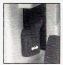
Pull the lever inside the vehicle to open the hood. It is located on the lower left side of the instrument panel.
