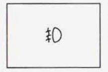
This light will come on when the fog lamps are in use. It will go out when the fog lamps are turned off.
