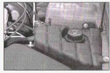
A low coolant level should be indicated by a CHECK COOLANT LEVEL message on the Driver Information Center. If it is, you may have a leak at the pressure cap or in the radiator hoses, heater hoses, radiator, water pump or somewhere else in the cooling system.
