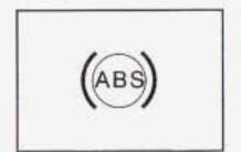
If there's a problem with the anti-lock brake system, this warning light will stay on. See Anti-Lock Brake System Warning Light on page 3-41.
