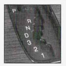
PARK (P): This position locks the front wheels. It's the best position to use when you start the engine because your vehicle can't move easily.
