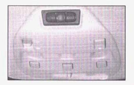
HomeLink<sup>®</sup>, a combined universal transmitter and receiver, provides a way to replace up to three hand-held transmitters used to activate devices such as gate operators, garage door openers, entry door locks, security systems and home lighting. Additional HomeLink<sup>®</sup> information can be found on the internet at www.homelink.com or by calling 1–800–335–3515.
