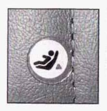
To assist you in locating the lower anchors for this child restraint system, each seating position with the LATCH system will have the LATCH system symbol on the seatback directly above the anchors.
