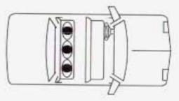
Your vehicle has the LATCH system. You'll find anchors (A) in all three rear seating positions.
