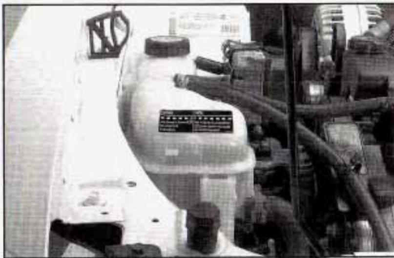
The engine coolant surge tank is located in the engine compartment on the passenger's side of the vehicle. See *Engine Compartment Overview* on page 5-12 for more information on location.
