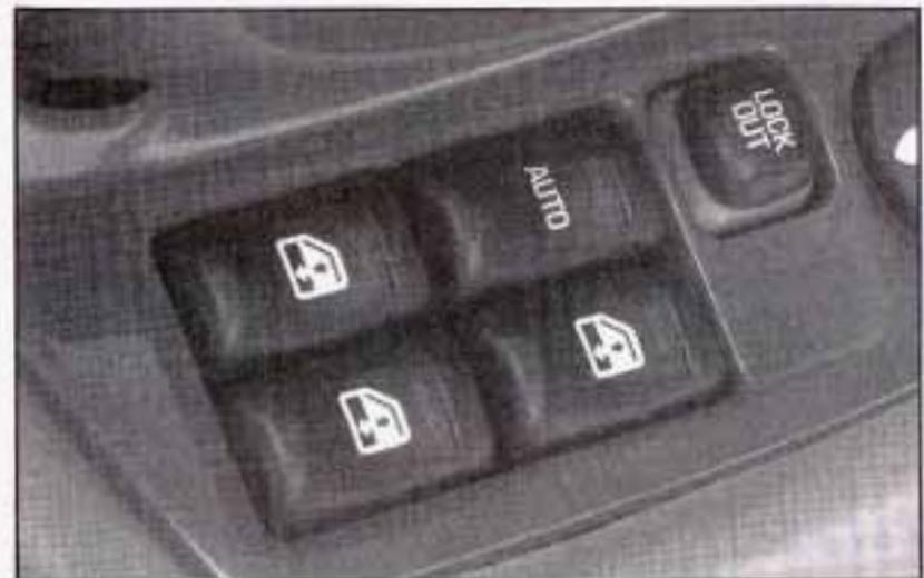
The power window switches are located on the armrest on the driver's door. In addition, each passenger door has a switch for its own window.
