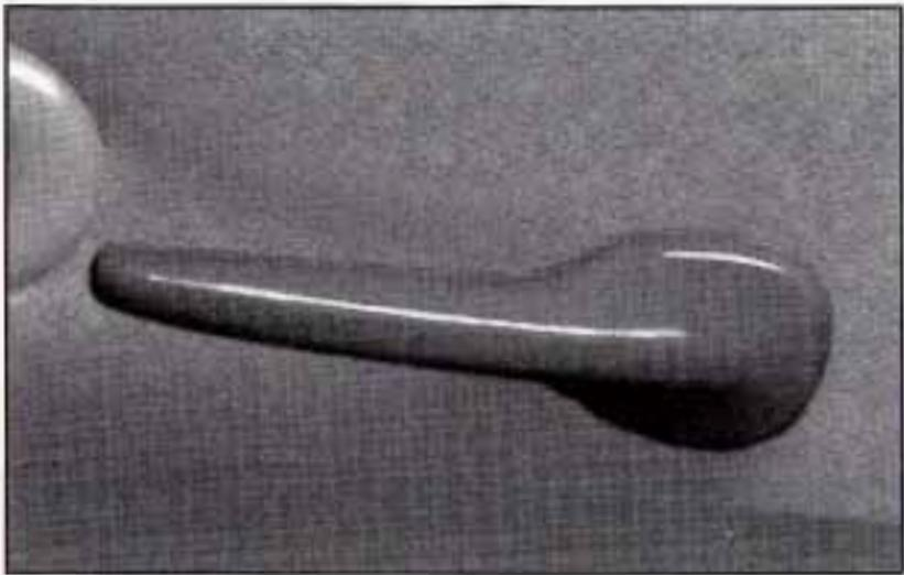
To adjust the seatback, lift the lever located on the outboard side of the seat and move the seatback to where you want it. Release the lever to lock the seatback. Pull up on the lever without pushing on the seatback, and the seatback will go to an upright position.
