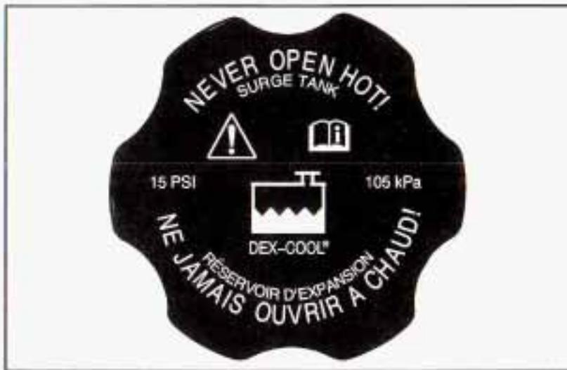
5. Then replace the pressure cap. Be sure the pressure cap is hand-tight and fully seated. See your dealer, if necessary.
