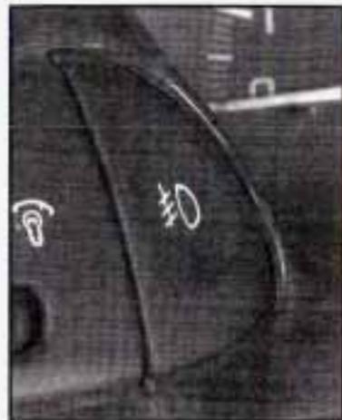
If your vehicle has this feature, the button for the fog lamps is located on the instrument panel, to the left of the steering wheel.
