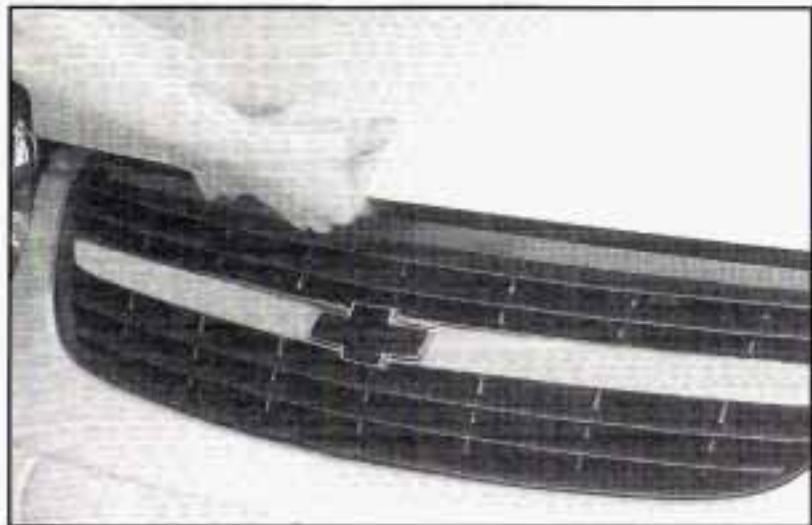
2. Then go to the front of the vehicle and lift the secondary hood release handle before lifting the hood.
