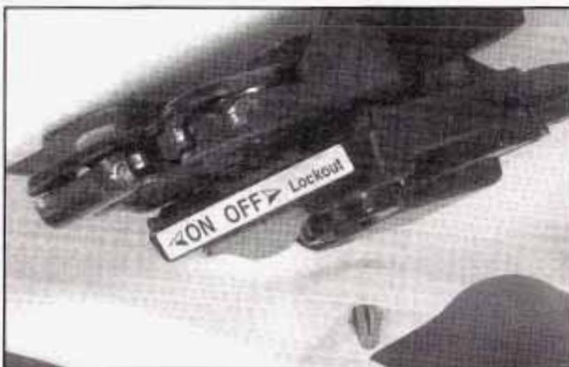
To turn the lockout on, slide the switch all the way to the left (ON). To turn the lockout off, slide the switch all the way to the right (OFF).
