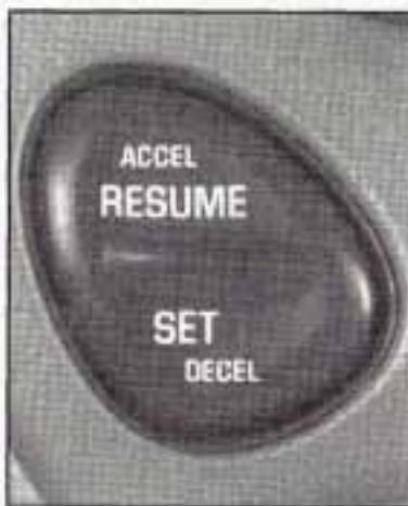
If your vehicle has cruise control, you can maintain a speed of about 25 mph (40 km/h) or more without keeping your foot on the accelerator. This can really help on long trips. Cruise control does not work at speeds below 25 mph (40 km/h).
