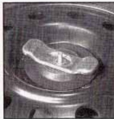
3. Turn the wing nut counterclockwise and remove it. Then lift off the adapter and remove the compact spare tire. See *Compact Spare Tire* on page 5-71 for more information about the compact spare tire.
