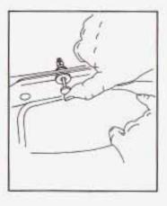
Push the flat end of the push-pin towards the retainer until it locks into place, making sure each is secure.
