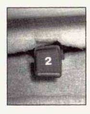
To unlatch the seat from the floor, pull up on the release lever labeled 2, located at the rear of the seat, and lift the rear of the seat up off the floor.
