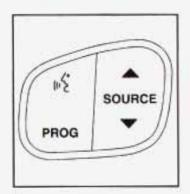
in ξ: If your vehicle is equipped with the steering wheel control buttons you can use them to interact with the OnStar<sup>®</sup> system.
