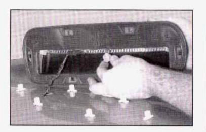
5. Reinstall the lens and tighten the screws.
