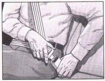
Pick up the latch plate and pull the belt across you. Don't let it get twisted. Push the latch plate into the buckle until it clicks.Pull up on the latch plate to make sure it is secure.
