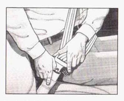
To unlatch the belt, just push the button on the buckle. The belt should go back out of the way.
