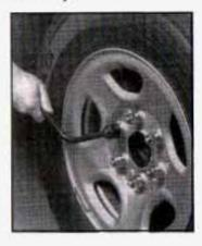
Use the wheel wrench to loosen all the wheel nuts. Turn the wheel wrench counterclockwise to loosen the wheel nuts. Don't remove the wheel nuts yet.
