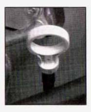
The engine oil dipstick has a yellow ring handle and is located in the engine compartment on the passenger's side of the vehicle. See Engine Compartment Overview on page 5-14 for more information on location.
