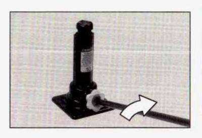
Turn the wheel wrench clockwise to raise the jack lift head to the lifting point.
