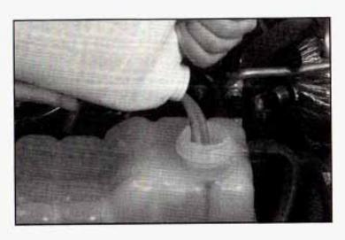
Then fill the coolant surge tank with the proper mixture, to the FULL COLD mark.
