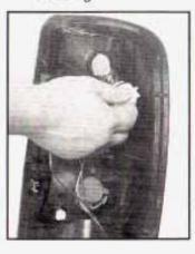
Pull the old bulb straight out from the socket.
