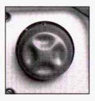
If your vehicle has this feature, the four-way control is located on the outboard side of the seat.
