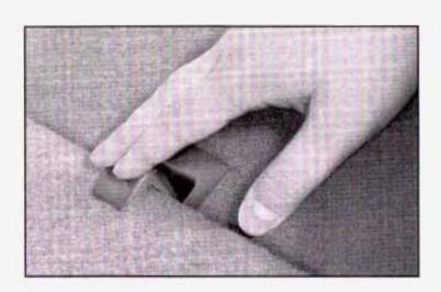
To create a load floor release the panels from the seatback by pushing forward on the latch. Then fold the panels back to cover the rear seat footwell area.
