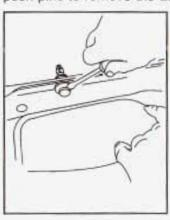
Insert a tool into the push-pin slot and pull downward until the push-pin snaps loose.
