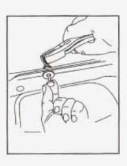
While continuing to pull downward on the push-pin, squeeze and turn the expandable end of the push-pin with a tool until it releases from the retainer. Notice: Operating your vehicle for extended periods without the front bumper lower air dam installed can cause improper air flow to the engine and may allow things like fog lamps or tow hooks on the front of your vehicle to be damaged. Always be sure to replace the front bumper air dam when you're finished off-road driving.
