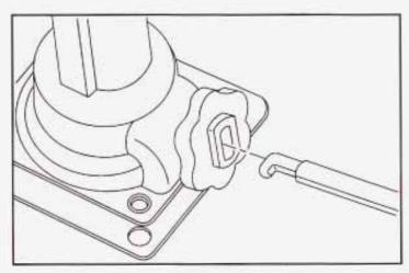
Attach the wheel wrench to the jack handle extensions (as needed). Attach the jack handle to the jack.
