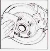
5. Remove any rust or dirt from the wheel bolts. mounting surfaces and spare wheel.
