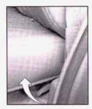
Pull the seatback release lever up and pull the seatback forward. Then fold it until it is flat.
