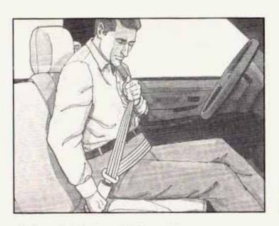
To make the lap part tight, pull down on the buckle end of the belt as you pull up on the shoulder belt.
