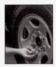
After mounting the spare, put the wheel nuts back on with the rounded end of the nuts toward the wheel. Tighten each wheel nut by hand using the wheel wrench until the wheel is held against the hub.
