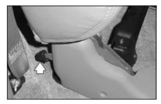
Yukon XL Denali: On the passenger side of Yukon XL Denali models, the lever at the base of the seat must be pulled up to release the seatback. Pull the seatback forward and fold it down until it is flat.
