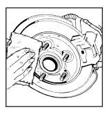
Remove any rust or dirt from the wheel bolts, mounting surfaces and spare wheel.
