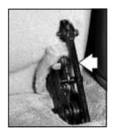
While holding the seat forward, pull the support rod out from the retainer clips and flip it down until it latches into place.
