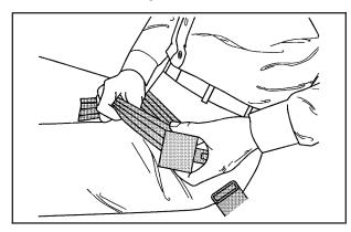
When you sit in the center position of a third row bench seat, you have a lap safety belt, which has no retractor. To make the belt longer, tilt the latch plate and pull it along the belt.
