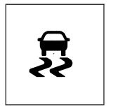
StabiliTrak® and part of the traction control system can be turned off or back on by pressing the StabiliTrak® button located on the instrument panel.
