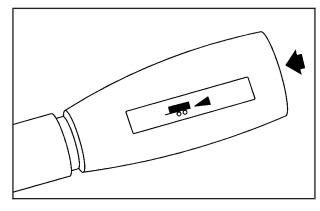
Your vehicle is equipped with a Tow/Haul mode. The button is located on the end of the column shift lever. You can use this feature to assist when towing or hauling a heavy load. See "Tow/Haul Mode" under *Towing a Trailer on page 4-50* for more information.
