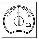
When your engine is not running, but the ignition is in RUN, this gage shows your battery's state of charge in DC volts.
