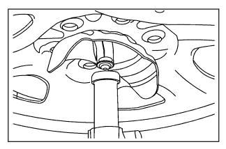
9. Position the center lift point of the jack under the center of the spare tire.
