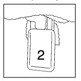
Unlatch the seat from the floor by pulling up on the lever labeled 2 located on the rear of the seat.
