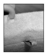
4. Pull on the release strap located in the lower middle of the seat to unlatch the seat from the floor and pull the seat out. Use one hand to pull the release strap and the other on the handle to pull the seat out.
