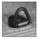
Your vehicle may be equipped with cargo tie downs in the rear cargo area that allow you to strap cargo in and keep it from moving inside the vehicle.
