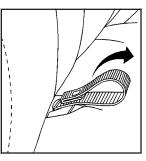
Pull up on the strap loop located in the center of the seat where the seatback and seat cushion meet and pull the seat cushion up. Then fold it forward.
