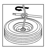
Use the wheel wrench hook which allows you to pull the hoist cable towards you to assist in reaching the spare tire.
