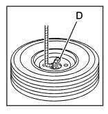
14. Tilt the retainer (D) at the end of the cable and pull it through the wheel opening. Pull the tire out from under the vehicle.
