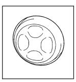
You can increase or decrease lumbar support in an area of the lower seatback with this control, located on the outboard sides of the front seat(s).
