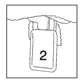
To unlatch the rear of the seat from the floor, pull up on the release lever labeled 2 at the rear of the seat, and lift the rear of the seat up from the floor.
