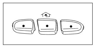
HomeLink<sup>®</sup>, a combined universal transmitter and receiver, provides a way to replace up to three hand-held transmitters used to activate devices such as gate operators, garage door openers, entry door locks, security systems, and home lighting. Additional HomeLink<sup>®</sup> information can be found on the Internet at www.homelink.com or by calling 1-800-355-3515.
