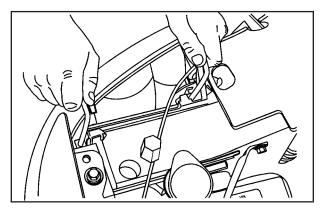
Remove the two pins on the top of the headlamp assembly. To remove them, turn the outer pin outward and pull it straight up. To remove the inner pin, turn it inward and pull it straight up.
