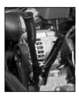
Connect the other end of the negative (–) cable to the remote negative (–) terminal, marked GND, on the vehicle with the dead battery.
