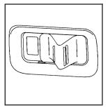
To unlock or lock the door from the inside, slide the manual lever forward or rearward.
