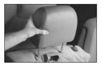
On the Yukon XL Denali models, you must remove the headrest and store it on the top of the seat cushion. Pull the headrest out from the seatback and slide the pins into the holes provided in the top of the seat cushion.
