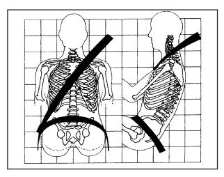
The lap part of the belt should be worn low and snug on the hips, just touching the thighs. In a crash, this applies force to the strong pelvic bones. And you will be less likely to slide under the lap belt. If you slid under it, the belt would apply force at your abdomen. This could cause serious or even fatal injuries. The shoulder belt should go over the shoulder and across the chest. These parts of the body are best able to take belt restraining forces.
