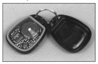
Insert a thin object, such as a coin, in the slot between the covers of the transmitter housing near the key ring hole. Remove the bottom by twisting the coin.
