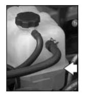
The coolant level should be at or above the FULL COLD mark. If it is not, you may have a leak at the pressure cap or in the radiator hoses, heater hoses, radiator, water pump or somewhere else in the cooling system.
