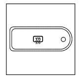
When this button is pressed, a defogger warms the driver's and passenger's outside rearview mirrors to help clear them of ice, snow, and condensation.
