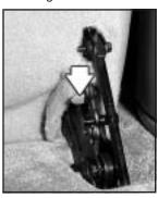
Pull the lever on the support rod bracket until it unlatches from the seat bracket.
