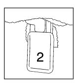
To unlatch the rear of the seat from the floor, pull up on the release lever labeled 2 at the rear of the seat and lift the rear of the seat up from the floor.
