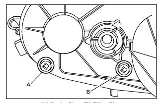
(A) Drain Plug (B) Filler Plug
