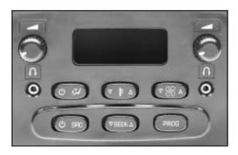
(Power): Press this button to turn the system on or off. The rear speakers will be muted when the power is turned on unless your vehicle is equipped with the Bose® audio system.
