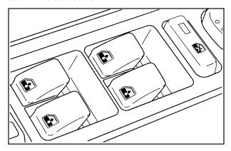
The driver's door has a switch for the passenger and rear windows as well. Your power windows will work when the ignition has been turned to ACCESSORY or RUN or when Retained Accessory Power (RAP) is active. See *Retained Accessory Power (RAP) on page 2-17*.
