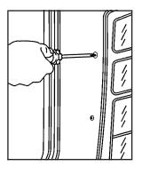
Remove the two screws from the taillamp assembly.
