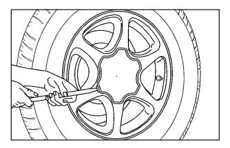
Remove the center cap by placing the chisel end of the wheel wrench in the slot on the wheel and gently pry the cap out.
