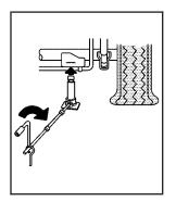
Rear Tire Flat: If the flat tire is on a rear tire of the vehicle, you'll need to use the jack handle (C) and both jack handle extensions (D). Attach the wheel wrench to the jack handle extensions. Attach the jack handle to the jack. Use the jacking pad provided on the rear axle.
