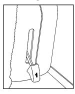
1. To return the seatback to an upright position, pull up on the release lever labeled 1 and then pull up on the seatback until it locks into the upright position.
