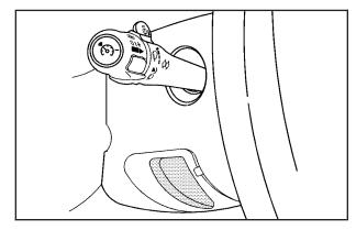
The tilt steering wheel lever is located on the lower left side of the column.
