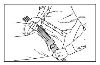
To make the belt shorter, pull its free end as shown until the belt is snug. Buckle, position and release it the same way as the lap part of a lap-shoulder belt. If the belt is not long enough, see *Safety Belt Extender on page 1-47*.
