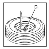
Tilt the retainer (D) at the end of the cable when the tire has been lowered, so it can be pulled up through the wheel opening.
