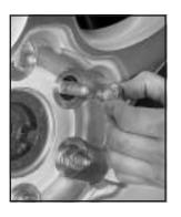
Put the wheel nuts back on with the rounded end of the nuts toward the wheel after mounting the spare. Tighten each wheel nut by hand. Then use the wheel wrench to tighten the nuts until the wheel is held against the hub.
