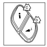
A 7: (Trip Information): Press this button to display the odometer, trip odometers, tire pressure for vehicles equipped with a tire pressure monitor, timer and engine hours.
