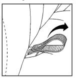
Pull up on the strap loop located in the center of the seat where the seatback meets the seat cushion. Pull the seat cushion up and fold it forward.
