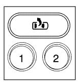
If your vehicle has this feature, the controls for the memory function are located on the driver's door.
