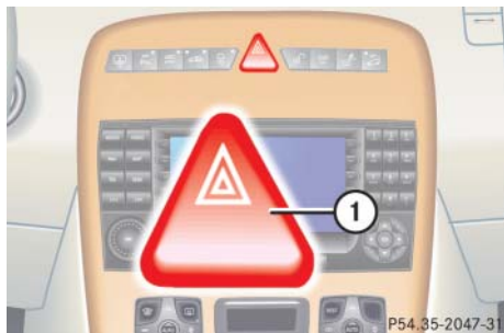
① Hazard warning flasher switch
