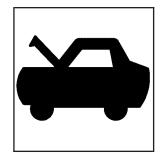
Pull the hood release handle with this symbol on it. It is located under the instrument panel on the driver's side of the vehicle.
