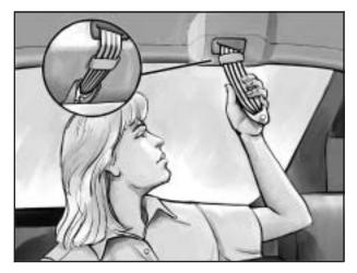
Remove the shoulder belt from its stowage location in the roof and pull it all the way down to the lap belt.
