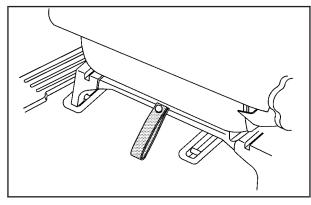
Pull the nylon strap behind the chair to release the rear hooks from the floor pins.
