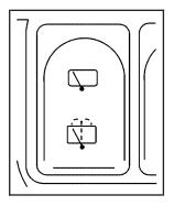
The rear window washer/wiper switch is located in the instrument panel switchbank. See Instrument Panel Switchbank on page 3-20.
