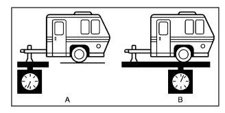
If you are using a weight-carrying or weight distributing hitch, the trailer tongue weight (A) should be 10 percent to 15 percent of the total loaded trailer weight (B). Do not exceed the maximum allowable tongue weight for your vehicle.
