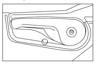
To adjust a seatback, pull up on the lever located on the outboard side of the driver's or front passenger's seats. Release the lever to lock the seatback where you want it. Push and pull on the seat to make sure it is locked into position.
