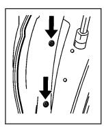
2. Remove the two screws on the inboard taillamp panel.
