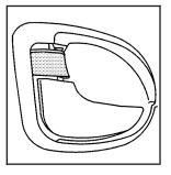
To unlock either manual locking front door from the inside, pull back on the manual lever. To lock either front door from the inside, push the manual lever forward.
