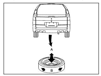
Make sure the tire is stored securely. Push, pull (A), and then try to turn (B) the tire. If the tire moves, use the folding wrench to tighten the cable.  Put back all tools as they were stored in the jack storage compartment and put the compartment cover back on.
