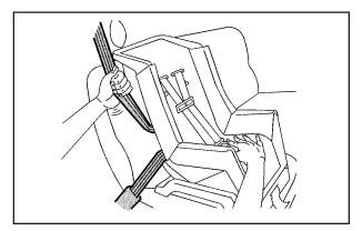
4. To tighten the belt, push down on the child restraint, pull the shoulder portion of the belt to tighten the lap portion of the belt and feed the shoulder belt back into the retractor. If you are using a forward-facing child restraint, you may find it helpful to use your knee to push down on the child restraint as you tighten the belt.
