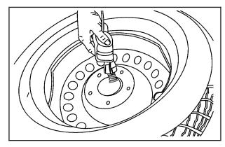
Tilt the retainer and slip it through the wheel opening to remove the spare tire from the cable.
