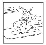
Make sure that the bench seat is angled so that the front hooks clear the floor pins. If the front legs are not attached correctly, the rear legs will not attach to the rear set of floor pins.
