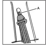
To move it down, push down on the button (A) and move the height adjuster to the desired position. You can move the height adjuster up by pushing up on the shoulder belt guide.
