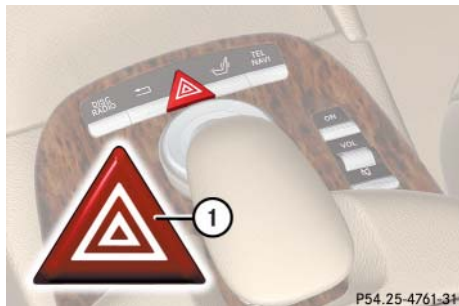
① Hazard warning flasher switch
