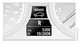
The remaining driving distance and the date for the next maintenance are displayed briefly with the ignition switched on. The first oil change displayed at approx. 1,200 miles/2,000 km signals that the break-in check is due.
