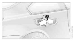
Place the fuel filler cap in the bracket attached to the fuel filler door.
