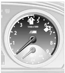
The advance warning field, arrow 1, and the red warning field, arrow 2, change depending on the engine temperature. As the engine temperature rises, the permissible engine speed also increases. Avoid allowing the engine speed to rise as far as the advance warning field whenever possible.
