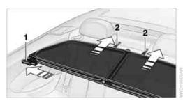
Guide the rear mounts 2 into the receptacles provided. Push the securing pin 3 on the left side into the appropriate opening until it snaps into place.
