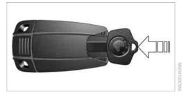
Remove the adapter from the holder in the glove compartment and slide the spare key into the adapter before use.
