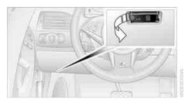
Components which are decisive for the exhaust-gas composition can be checked via the OBD socket with a device.
