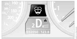
▲ This symbol means that a Check Control message has been generated. The symbol remains visible even if the Check Control message has been hidden after a short time. The combinations of warning lamps and text messages are stored and can be viewed later, also refer to page 75.
