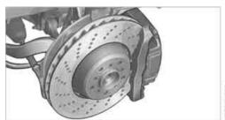
Your BMW M6 has a high-performance brake system with perforated compound brake rotors.
