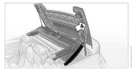
Do not carry out the next operation, raising top ends, until the top has been swung forward, otherwise damage can occur.
