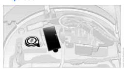
The M Mobility System is located in the luggage compartment under the floor panel flap.
