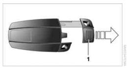
Press button 1 to unlock the key.
