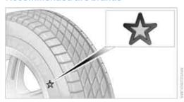
BMW recommends particular tire brands for each tire size. You can recognize these from the clearly visible BMW marking on the tire sidewall. With proper use, these tires meet the highest standards for safety and handling characteristics.
