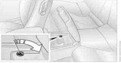
Turn the key to the right, refer to illustration, until the key slot points in the direction of travel and then remove:
