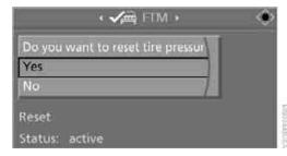
The message "resetting FTM ..." is displayed for a few seconds. The warning lamp in the instrument cluster lights up yellow for a few seconds.
