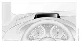
Only clean the cover of the Head-Up Display with a soft, nonabrasive cloth or with a display cleaning cloth; otherwise, you may damage it. ◀
