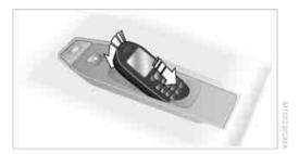
From radio readiness or with the steering unlocked the mobile phone's battery is charged.
