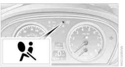
From radio readiness, refer to page 59, the warning lamp lights up briefly, indicating the operational readiness of the entire airbag system and the safety belt tensioners.
