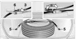
Convertible: hook the belt into the lashing eyes 5 and 7 and lay it in the belt guide of the lid which runs offset.
