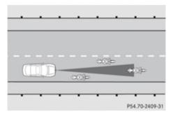
Because of their narrow profile, the vehicles traveling near the outer edges of the lane have not yet been detected by the DISTRONIC Plus. There will be insufficient distance to the preceding vehicles.
