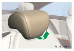
Adjust the head restraint to the desired position by pushing or pulling on the upper edge of the head restraint cushion.
