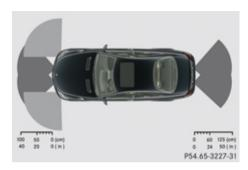
Due to the sensors' broad detection range, it is possible that the Park Assist also detects and issues a warning for obstacles in the ground, e.g. sewer canal covers, rails, bumps in the road or gutters or obstacles moving upward quickly, e.g. rolling garage doors.
