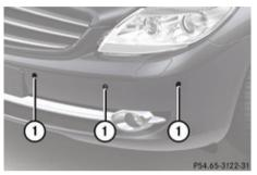
(1) Sensors in the front bumper (Only visible without DISTRONIC Plus)
