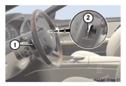
Steering wheel gearshift control (example illustration)
