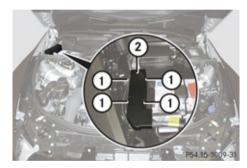
Example illustration fuse box on passenger side
