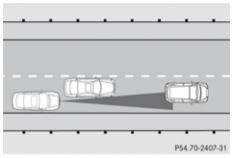
A vehicle traveling in your lane but offset from your direct line of travel may not be detected by the DISTRONIC Plus. There will be insufficient distance to the preceding vehicle.
