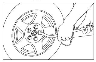
If your vehicle has plastic wheel covers, use the wheel wrench to loosen the plastic wheel nut caps.
