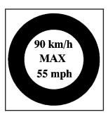
15. If the flat tire was able to inflate to the recommended inflation pressure, remove the maximum speed label from the sealant canister (B) and place it in a highly visible location.
