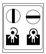
The rear door security locks are located on the inside edge of each rear door. You must open the rear doors to access them. The label showing lock and unlock positions is located near the lock.
