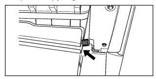
Lower the glove box door by pressing in on each side and lowering from the track.
