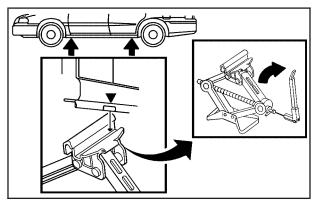
Position the jack lift head at the rear jack location nearest the rear tire. The rear location is about 4 inches (10 cm) in front of the rear wheel opening.
