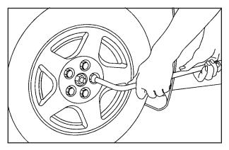
2. If your vehicle has plastic wheel covers, use the wheel wrench to loosen the plastic wheel nut caps.
