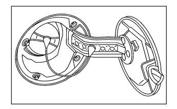
The tethered fuel cap is located behind a hinged fuel door on the passenger side of the vehicle.
