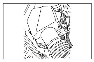
To inspect or replace the filter, remove the screws that hold the cover on and lift off the cover. Be sure to reinstall the cover tightly.
