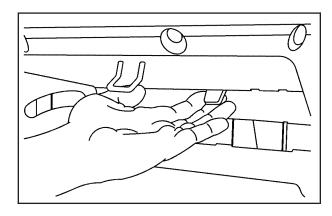
Pull the tab at the back of the glove box toward you and open the passenger compartment air filter door downward.
