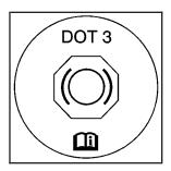
The brake master cylinder and, on manual transmission vehicles, the clutch hydraulic system use the same reservoir filled with DOT 3 brake fluid.
