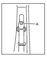
Press the release button (A) and move the height adjuster to the desired position. The adjuster can be moved up by pushing up on the shoulder belt guide.
