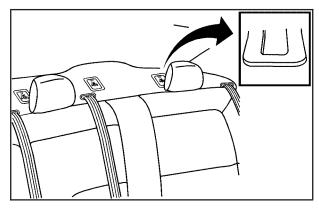
Do not secure a child restraint in a position without a top tether anchor if a national or local law requires that the top tether be attached, or if the instructions that come with the child restraint say that the top tether must be attached.
