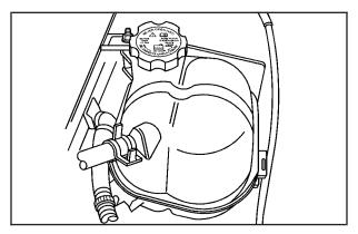
The coolant surge tank is located in the engine compartment on the driver's side of the vehicle. See *Engine Compartment Overview on page 5-12* for more information on location.
