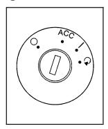
The ignition switch has four different positions.
