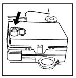
Locate the remote positive (+) terminal which is located under a red tethered cap on the engine compartment fuse block. Lift the cap to access the terminal.
