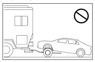
The vehicle cannot be dolly towed, but can be dinghy towed. See "Dinghy Towing" earlier in this section.
