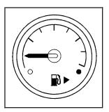
The fuel gage shows about how much fuel the vehicle has left.
