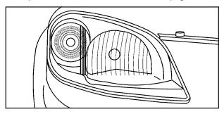
Record the distance from the ground to the aim dot on the low-beam headlamp.
