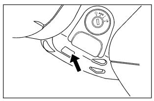
Remove the cover from the bottom of the steering column.
