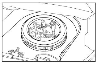
2. Lift the trunk liner to access the spare tire and tools.
