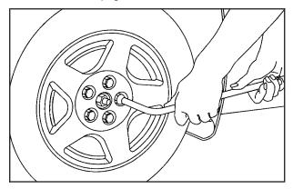
3. If your vehicle has plastic wheel covers, use the wheel wrench to loosen the plastic wheel nut caps.
