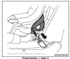
Route the seat belt tongue through the child restraint and insert it into the buckle until you hear and feel the latch engage. Be sure to follow the child restraint manufacturer's
