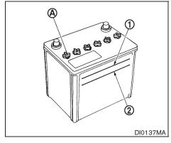
Check the fluid level in each cell. It should be between the UPPER LEVEL (1) and LOWER LEVEL (2) lines.
