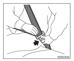
Unfastening the seat belts To unfasten the seat belt, push the button on the buckle. The seat belt automatically retracts.
