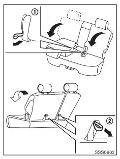
To fold down the seatback of each rear seat, pull the strap (1) or (2).
