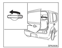
To open the back door, unlock it and pull the handle.
