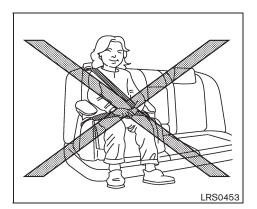
Make sure the child's head will be properly supported by the booster seat or vehicle seat. The seatback must be at or above the center of the child's ears. For example, if a low back booster seat (1) is chosen, the vehicle seatback must be at or above the center of the child's ears. If the seatback is lower than the center of the child's ears, a high back booster seat (2) should be used.
