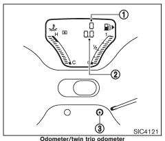
Odometer/twin trip odometer
