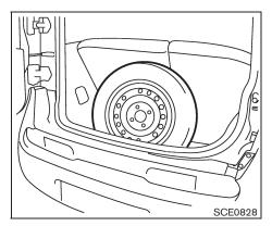
Securely store the damaged tire in the cargo area as illustrated.
