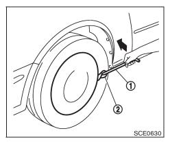
Removing wheel cover (if so equipped)
