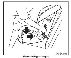
Remove any additional slack from the seat belt; press downward and rearward firmly in the center of the child restraint with your knee to compress the vehicle seat cushion and seatback while pulling up on the seat
