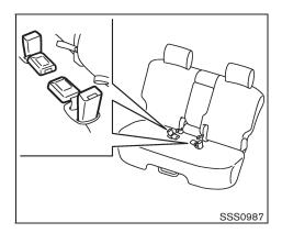
Stow seat belt buckles by pushing the seat belt buckles into seat pockets.
