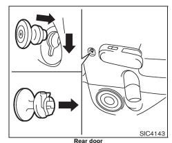
The utility hooks can be attached to the holes as illustrated.
