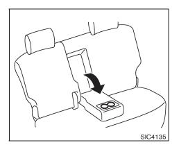
Rear (if so equipped) Pull the armrest forward until it is horizontal.
