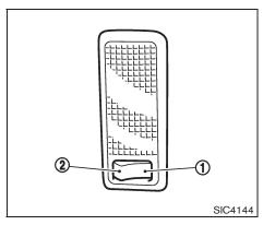
When the switch is in the ON position (1), the light illuminates while the back door is opened. When the back door is closed, the light will turn off.
