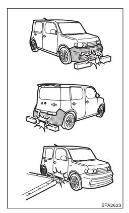
The Krōm models have unique front and rear bumpers and side sill extensions. These parts are close to the ground and may be damaged if they contact objects such as curbs, parking blocks, etc.
