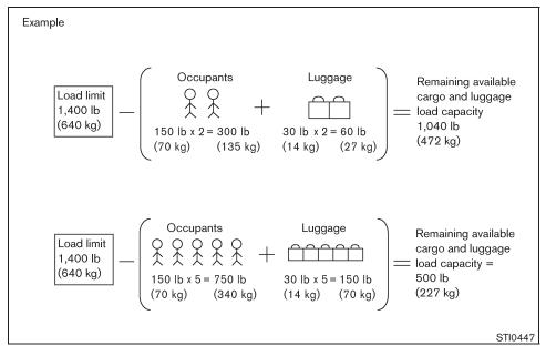
Steps for determining correct load limit
