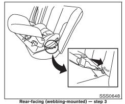
3. Secure the child restraint anchor attachments to the LATCH lower anchors. Check to make sure the LATCH attachment is properly attached to the lower anchors.
