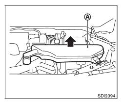
Removing the resonator
