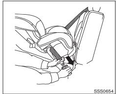
Rear-facing — step 2 Route the seat belt tongue through the child restraint and insert it into the buckle until you hear and feel the latch engage. Be sure to follow the child restraint manufacturer's instructions for belt routing.
