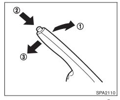
To apply: Pull the parking brake lever up (1).
