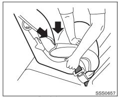
Rear-facing — step 5 Remove any additional slack from the child restraint; press downward and rearward firmly in the center of the child restraint with your hand to compress the vehicle seat cushion and seatback while pulling up on the seat belt.
