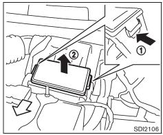
To remove the air cleaner filter, push the tabs 1 and pull the filter upward 2.
