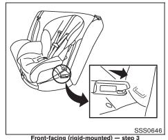
The back of the child restraint should be secured against the seatback. If necessary, remove the headrest to obtain the correct child restraint fit. (See "HEAD RE-STRAINTS" earlier in this section.)
