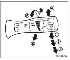
Pull the lever toward you (5) to operate the washer. Then the wiper will also operate several times.
