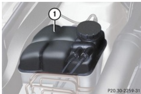
① Coolant expansion tank
