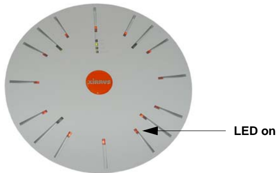
Figure 59. LEDs are Switched On
