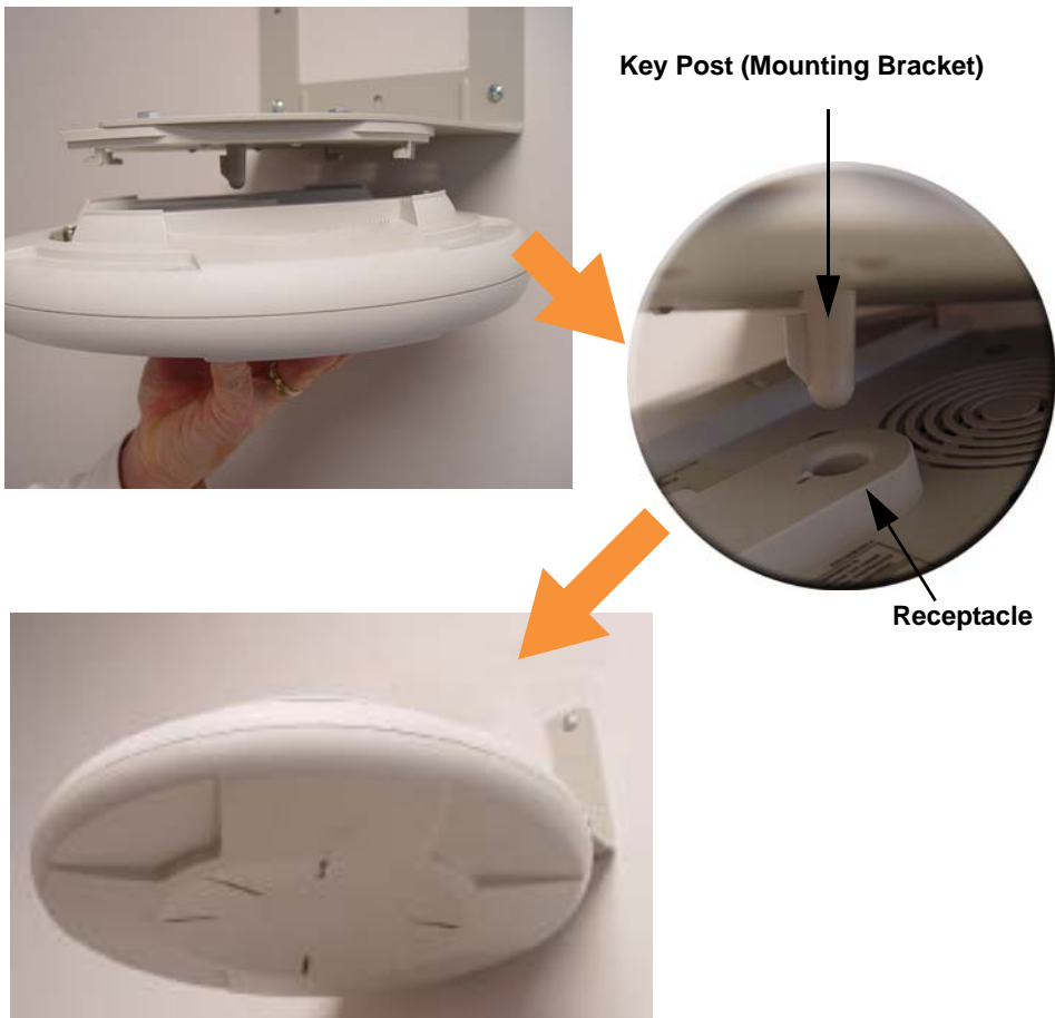
Figure 55. Mounting the Array on a Wall
