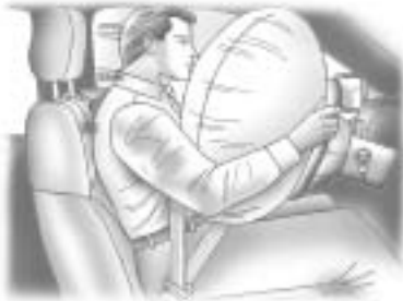
The driver's frontal airbag is in the middle of the steering wheel.
