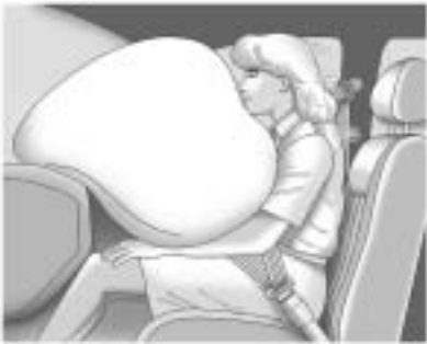
The right front passenger frontal airbag is in the instrument panel on the passenger side.
