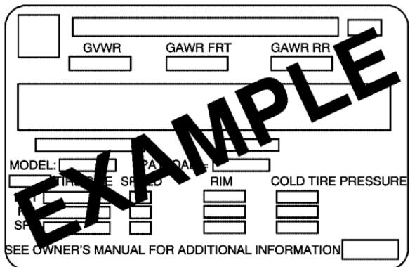
A vehicle specific Certification/Tire label is found on the rear edge of the driver's door, or on the vehicle's center pillar (B-pillar).
