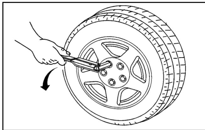
2. Using the wheel wrench, loosen all the wheel nuts on the rear tire. Do not remove them yet.
