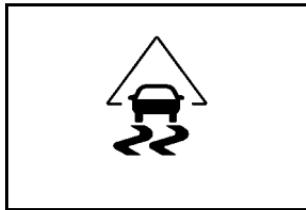
When this light is on and either the SERVICE TRACTION or TRACTION OFF message is displayed, the system will not limit wheel spin.
