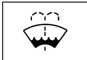
Open the cap with the washer symbol on it. Add washer fluid until the tank is full. See *Engine Compartment Overview* on page 6-16 for reservoir location.
