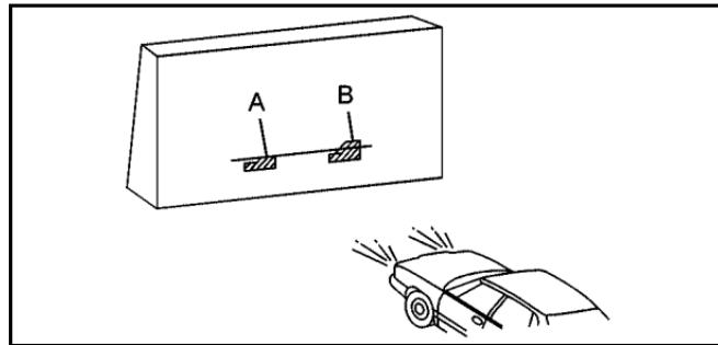
The top edge of the cut-off should be positioned at the bottom edge of the horizontal tape line.
