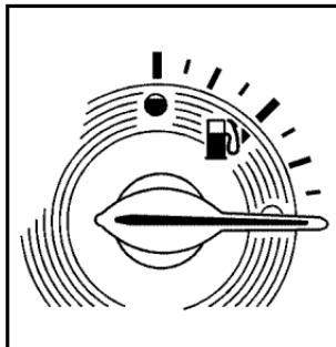
The fuel gauge indicates about how much fuel is left in the fuel tank.
