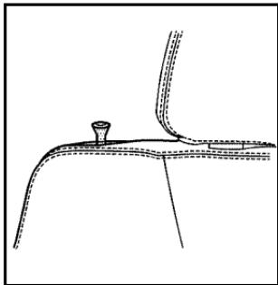
5. Pull up on the knob located on the top of the seatback on the outboard side to release the seatback.
