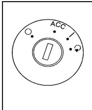
The ignition switch has four different positions.
