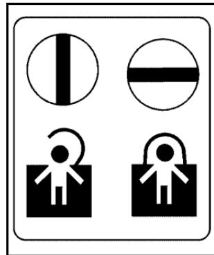
On vehicles with this feature, the rear door security locks are located on the inside edge of each rear door. You must open the rear doors to access them.
