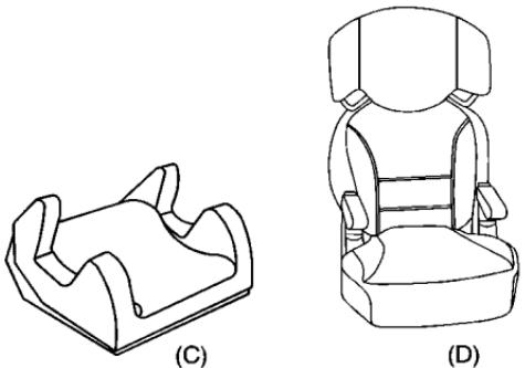
A booster seat (C-D) is a child restraint designed to improve the fit of the vehicle's safety belt system. A booster seat can also help a child to see out the window.
