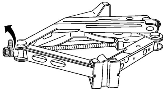
Turn the plastic wheel nut counterclockwise to loosen the wheel wrench from the jack.
