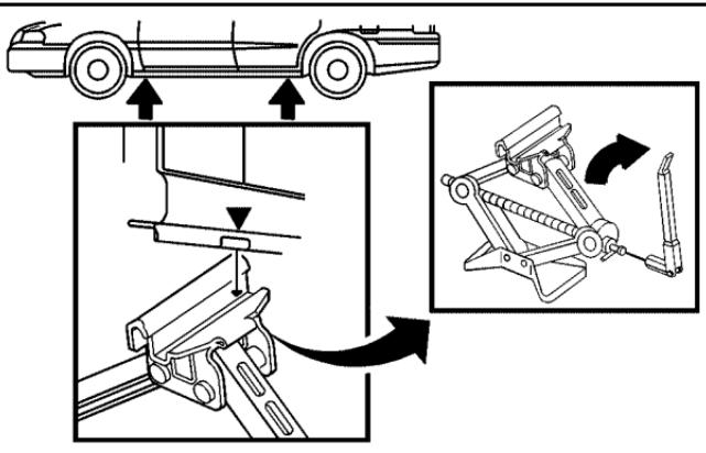
3. Position the jack on the front position and raise the jack lift head to fit over the car flange under the down arrow markings on the rocker panel.
