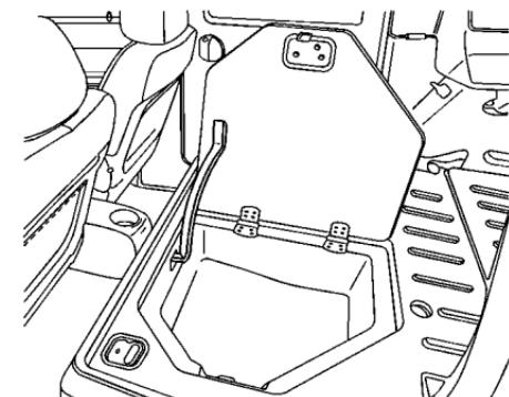
The vehicle may have two storage bins located in the rear of the vehicle. Pull up on the handles to open and lift the lid. Use the key to lock/unlock the bins.
