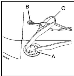
5. Route the loop end of the strap (C) through one of the cargo tie-downs (A) located in the rear of the vehicle.
