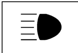
This indicator light appears on the instrument panel cluster when the high beams are on.
