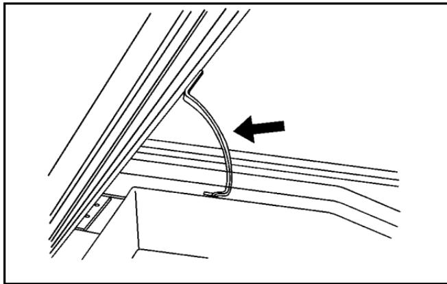
There is a rod that hooks into place to prop open the lid. Push the rod towards the lid to unhook it and lower the lid.
