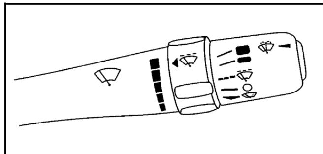
The windshield wiper lever is on the right side of the steering wheel.
