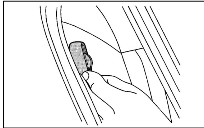
1. Pull the elastic cord out from between the edge of the seatback and the interior body to remove the guide from its storage clip.
