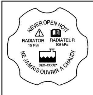
1. Remove the pressure cap when the cooling system, including the pressure cap and upper radiator hose, is no longer hot.
