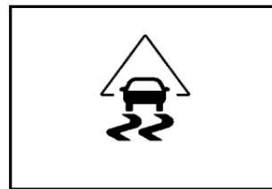
This indicator comes on whenever the vehicle StabiliTrak® is actively working.
