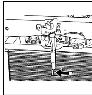
2. Then go to the front of the vehicle and push the secondary hood release lever to the left. It is located under the front center of the grille.
