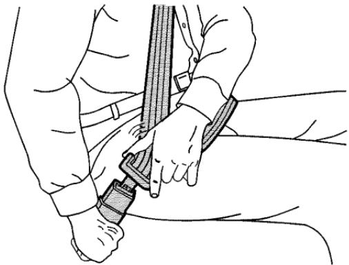
3. Push the latch plate into the buckle until it clicks. Pull up on the latch plate to make sure it is secure. If the belt is not long enough, see *Safety Belt Extender on page 2-34*. Position the release button on the buckle so that the safety belt could be quickly unbuckled if necessary.
