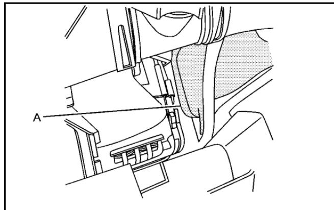
When the engine is cold, the coolant level should be at the COLD FILL (A) line or a little higher. The COLD FILL line is near the bottom of the tank and sticks out from the rear of the tank.
