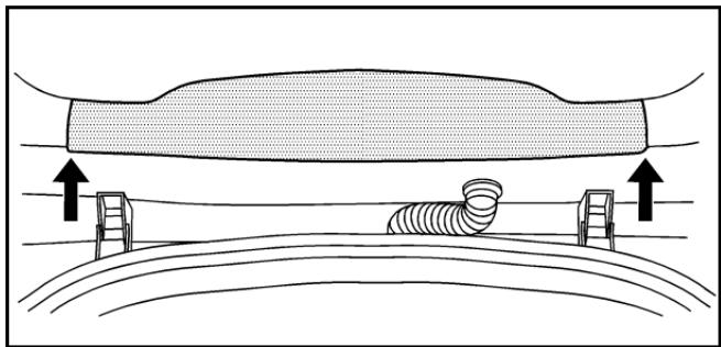
2. Remove the center trim located near the top of the liftgate.
