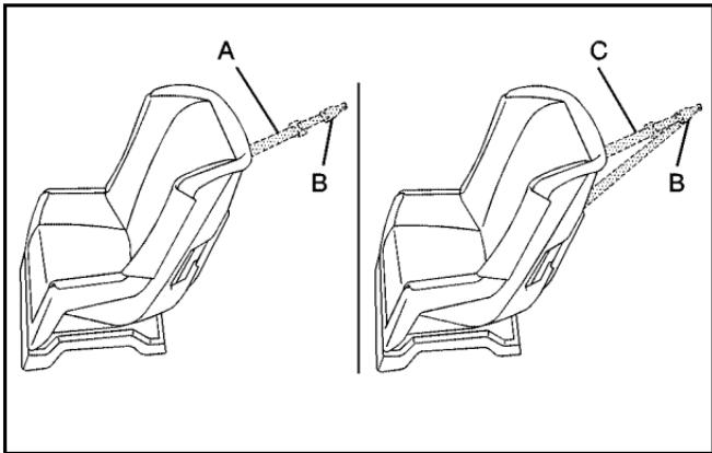
Your child restraint may have a single tether (A) or a dual tether (C). Either will have a single attachment (B) to secure the top tether to the anchor.
