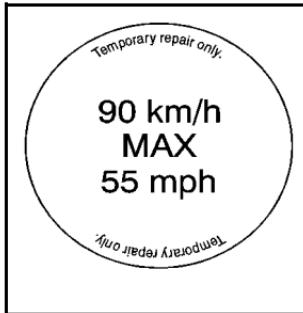
16. If the flat tire was able to inflate to the recommended inflation pressure, remove the maximum speed label from the sealant canister and place it in a highly visible location. The label is a reminder not to exceed 55 mph (90 km/h) until the damaged tire is repaired or replaced.
