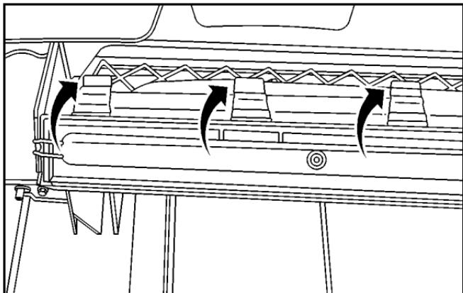
3. Pull the three tabs of the filter access door down and open the access door downward.
