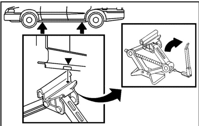
3. Position the jack and raise the jack lift head to fit over the car flange under the down arrow markings on the rocker panel.
