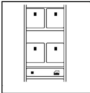
On vehicles with power windows, the switches are on each of the side doors. The driver door also has switches that control the passenger and rear windows.
