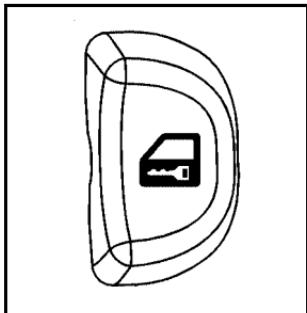
The power door lock switches are located on the driver's and front passenger's door next to the door handle.
