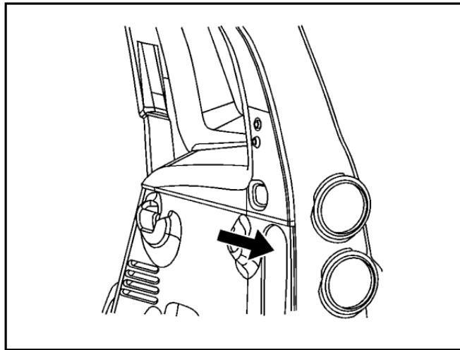
The vehicle may have a power plug connector located in the rear cargo area on the passenger side behind the service panel. The power connector wiring can be accessed by removing the service panel to begin installation.
