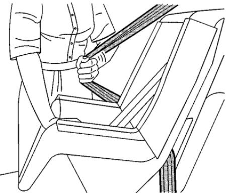
4. Pull the rest of the shoulder belt all the way out of the retractor to set the lock.
