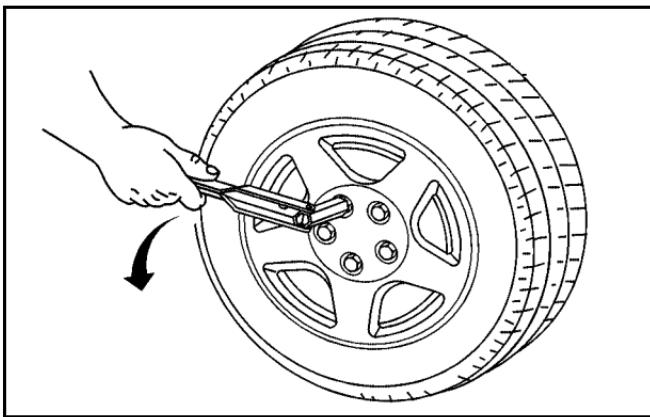
2. Using the wheel wrench, loosen all the wheel nuts.
