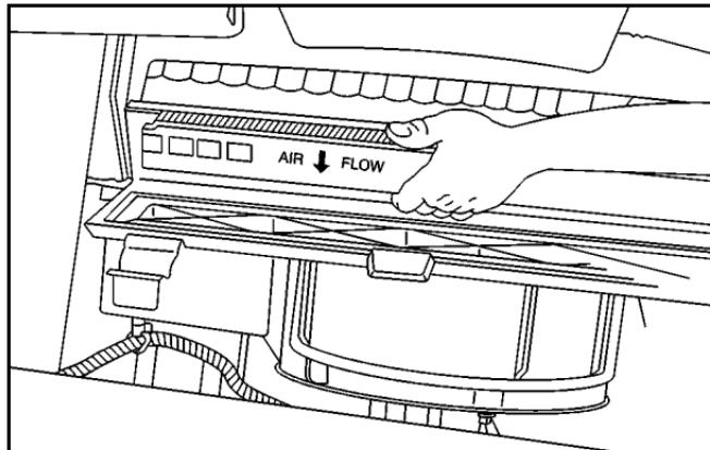
4. Pull the filter out, keeping it upwards.
