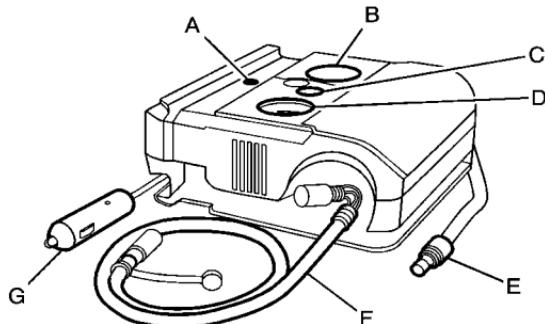
When using the tire sealant and compressor kit during cold temperatures, warm the kit in a heated environment for 5 minutes. This will help to inflate the tire faster.
