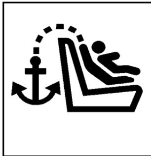
To assist you in locating the top tether anchors, this symbol is located next to each top tether anchor.
