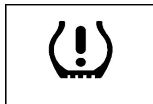
When a low tire pressure condition is detected, the TPMS turns on the low tire pressure warning light located on the instrument panel cluster.
