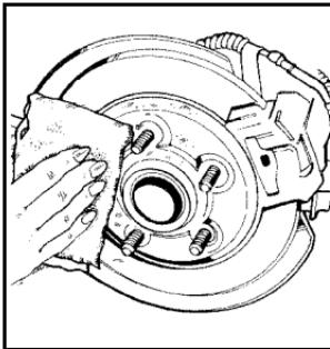
7. Remove any rust or dirt from the wheel bolts, mounting surfaces, and wheel.
