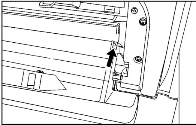
2. Press both glove box stops outward to let the glove box drop open completely.
