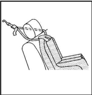
If the position you are using has an adjustable headrest or head restraint and you are using a dual tether, route the tether around the headrest or head restraint.
