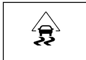
This light flashes while the traction control system is limiting wheel spin.
