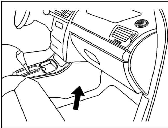
The floor console fuse block is located on the passenger side of the floor console behind the forward panel. The panel has four clips, one in each corner. Pull the panel to disconnect the four clips, and access the fuses. Use the fuse puller to remove fuses.
