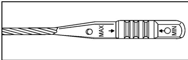
If the oil is below the MIN (minimum) mark, add at least one quart/liter of the recommended oil. This section explains what kind of oil to use. For engine oil crankcase capacity, see *Capacities and Specifications* on page 6-125.
