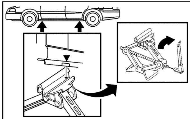
3. Position the jack on the rear position and raise the jack lift head to fit over the car flange under the down arrow markings on the rocker panel.
