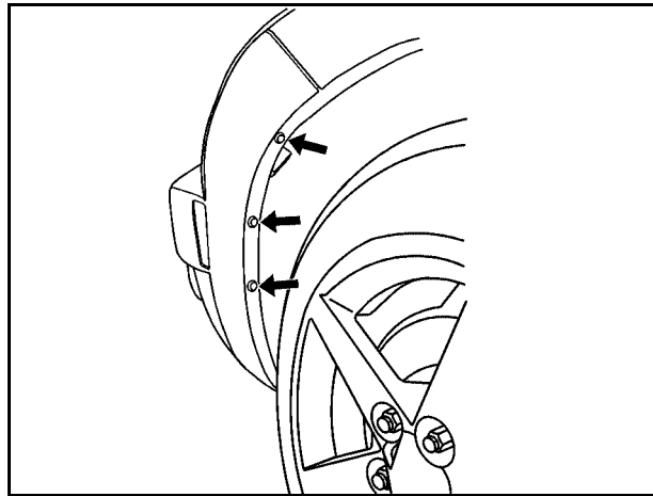
2. Remove the fasteners located on the wheel liner.
