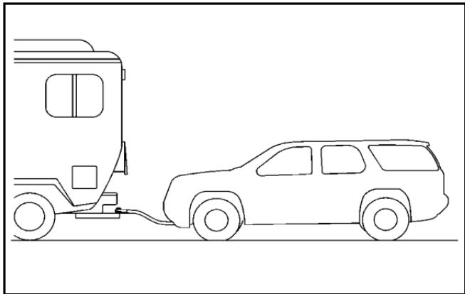
Use the following procedure to dinghy tow the vehicle from the front with all four wheels on the ground:
