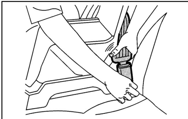
4. Push the latch plate into the buckle until it clicks. Position the release button on the buckle so that the safety belt could be quickly unbuckled if necessary.
