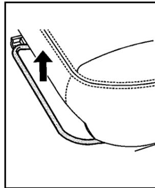
1. Lift the bar under the seat to unlock the seat.
