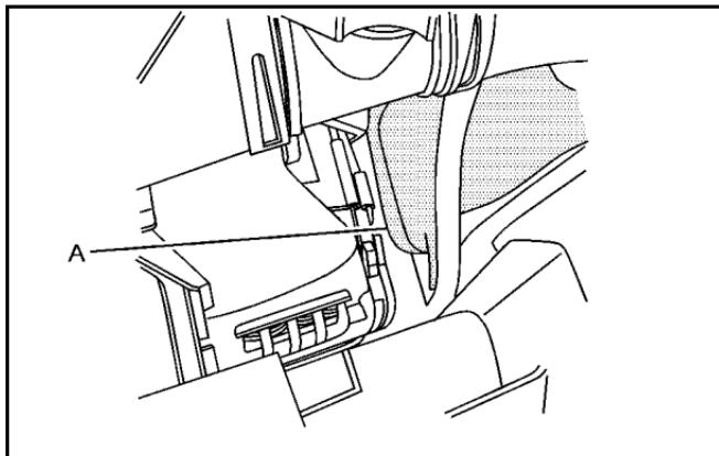
5. Then fill the coolant recovery tank to the COLD FILL (A) line.
