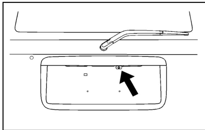
The area displayed by the camera is limited and does not display objects that are close to either corner or under the bumper. The area displayed can vary depending on vehicle orientation or road conditions. The distance of the image that appears on the screen differs from the actual distance.
