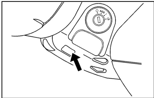
2. Remove the cover from the bottom of the steering column.
