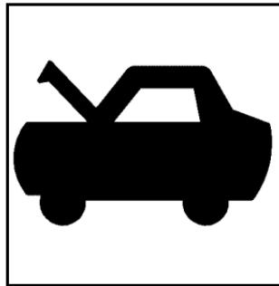
1. Pull the interior hood release lever with this symbol on it. It is located to the left of the instrument panel on the driver's side of the vehicle.
