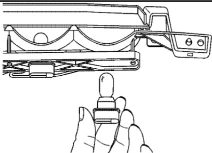
4. Pull the old bulb straight out of the bulb socket.
