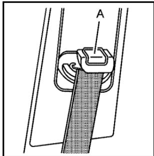
Push down on the release button (A) and move the height adjuster to the desired position. The adjuster can be moved up by pushing the release button up on the shoulder belt guide.
