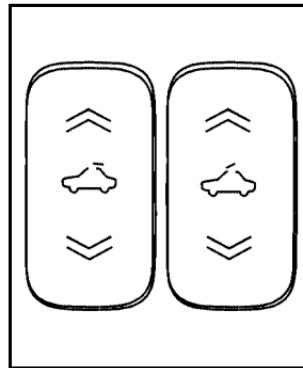
The switches that operate the sunroof are located in the headliner.
