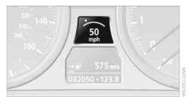
The car's current speed is stored. It is displayed on the speedometer and briefly in the instrument cluster.
