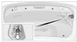
Take the warning triangle out of its holder, refer to page 238. Unscrew the holder using the screwdriver from the onboard vehicle tool kit.
