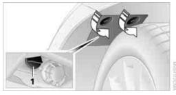
Rotate turn signal bulb socket 1 to the left and remove.
