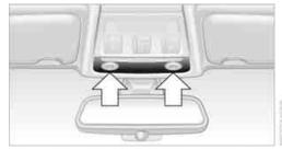
2. Insert the screwdriver into the openings on each side to press the clips.
