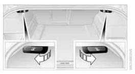
The unlocked rear seat backrest moves forward slightly. Fold the backrest forward by the head restraint.
