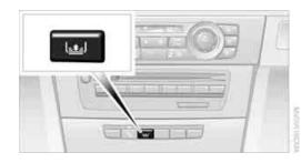
Tap the button in the center console to raise or lower the roller sun blind.
