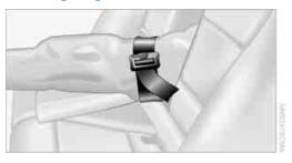
After loading, secure the ski bag and its contents. Tighten the retaining strap on the tensioning buckle for this purpose.
