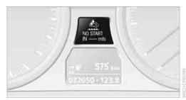
Even if the display indicates -- mls, the engine continues running if it is not switched off and if all other requirements continue to be met, e.g. a sufficient supply of fuel.
