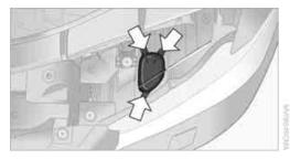
3. Release the wire bracket from the anchor, see arrow, and fold it up.
