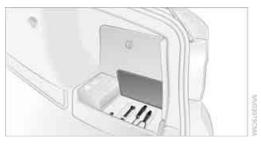
The onboard vehicle tool kit is stored in a compartment on the right-hand side of the cargo area. Remove the cover.
