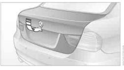
Press the button, see arrow, or the button on the remote control for a longer period. The trunk lid will open slightly. It can now be swung upwards.
