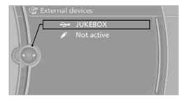
Playback begins with the first track. When an Apple iPhone is connected via the snap-in adapter and an audio device is connected to the AUX-IN port at the same time, the audio signal of the AUX-IN port is played.
