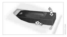
To remove the snap-in adapter: Press button 1.
