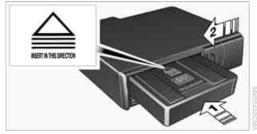
Insert the CD magazine all the way in the direction of arrow **1** and close the cover, arrow **2**.
