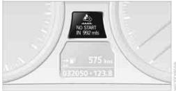
After refilling, the reserve display continues to be displayed after the engine is started. It goes out after the vehicle has been driven for several minutes.
