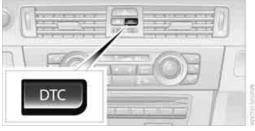
Press the button; the indicator lamps for DTC in the instrument cluster come on.
