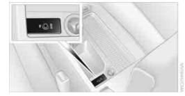
Connection for audio playback: TRS connector 1/8 in/3.5 mm
