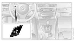
This symbol on the Control Display and an acoustic signal indicate that the voice activation system is ready to receive spoken commands.
