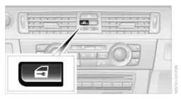
This button serves to unlock or lock doors and the trunk lid/tailgate, but does not activate the anti-theft system. The fuel filler flap remains unlocked.
