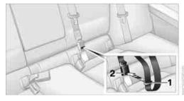
Insert the latch plate at the end of the belt into the specially designated fixture on the rear window shelf.
