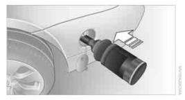
The reservoir is full when the filling level in the bottle stops changing. It is not possible to overfill the reservoir. Pull back the bottle, see arrow, and unscrew it.
