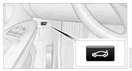
Press the button: the trunk lid/tailgate opens unless it has been locked.
