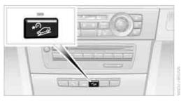
Press the button; the LED lights up. When the vehicle is being braked automatically, the LED flashes.
