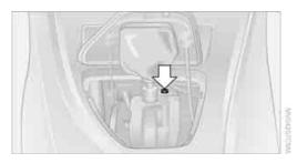
Using the screwdriver from the onboard vehicle tool kit, refer to page 229, press the red lever while moving the selector lever to the desired position.
