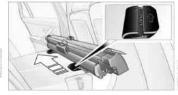
Slide the casing into the guides on the backs of the seat backrests.
