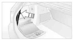
The warning triangle is located behind the lefthand trim panel in the cargo area. Press the tab to take it out.
