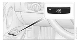
With the safety switch, you can prevent the rear windows from being opened or closed via the switches in the rear passenger area, by children, for example. When the safety function is switched on, the LED comes on.
