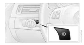
The parking lamps or low beams must be switched on for the fog lamps to operate. The green indicator lamp in
