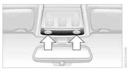
2. Insert the screwdriver into the openings on each side to press the clips.
