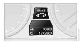
The remaining driving distance and the date of the next scheduled service are displayed briefly immediately after you start the engine or switch on the ignition.
