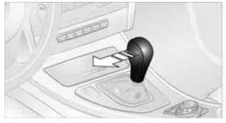
Move selector lever from position D toward the left into the M/S shifting slot:
