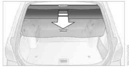
Press the button: the roller cover is raised. Before closing the rear window or tailgate, press the roller cover downward until it engages.
