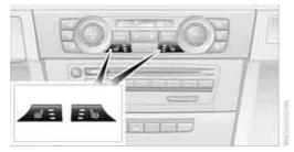
Press the button once per temperature level. Three LEDs indicate the highest temperature.
