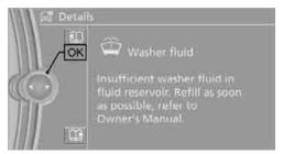
You can call up more information on the Control Display, e.g. on the cause of a malfunction and on how to respond, via Check Control, refer to page 77.
