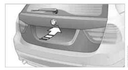
Press the button, see arrow, or the button on the remote control for a longer period. The tailgate will open slightly. It can now be swung upwards.
