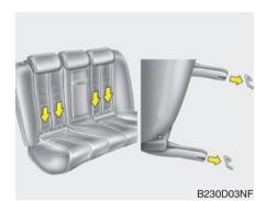
LATCH anchors have been provided in your vehicle. The LATCH anchors are located in the left and right outboard rear seating positions. Their locations are shown in the illustration. There is no LATCH anchor provided for the center rear seating position.
