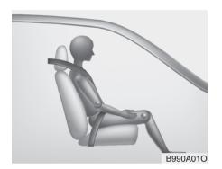
When an adult is seated in the front passenger seat, if the PASS AIR BAG "OFF" indicator is on, turn the ignition switch to the LOCK position and ask the passenger to sit properly (sitting upright with the seat back in an upright position, centered on the seat cushion with their seat belt on, legs comfortably extended and their feet on the floor). Restart the engine and have the person remain in that position. This will allow the system to detect the person and to enable the passenger air bag.
