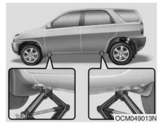
7. Place the jack at the front or rear jacking position closest to the tire you are changing. Place the jack at the designated locations under the frame. The jacking positions are plates welded to the frame with two tabs and a raised dot to index with the jack.
