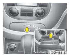
The front ashtray may be opened by pressing the ashtray lid. To clean the ashtray, the plastic receptacle should be removed by lifting the plastic ash receptacle upward and pulling it out.
