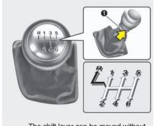
The shift lever can be moved without pulling the ring (1).
