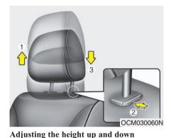
To raise the headrest, pull it up to the desired position (1). To lower the headrest, push and hold the release button (2) on the headrest support and lower the
