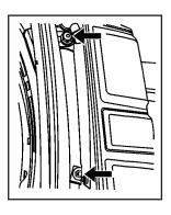
Remove the two inboard nuts from the inside of the taillamp assembly.
