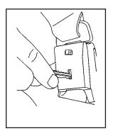
To do this, press the tip of a key into the release hole of the safety belt buckle while pulling up on the safety belt.
