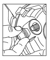
Put the wheel nuts back on with the rounded end of the nuts toward the wheel. Tighten each wheel nut by hand until the wheel is held against the hub.
