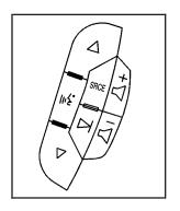
If equipped, these controls are located on the right side of the steering wheel.
