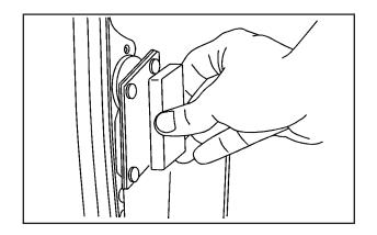
To open the rear portion of a 60/40 door from the outside, pull the handle on the side of the rear door and pull the door toward you.
