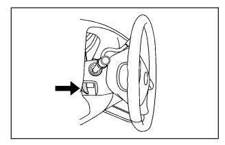
For vehicles with a tilt steering wheel, the lever is located on the left side of the steering column.
