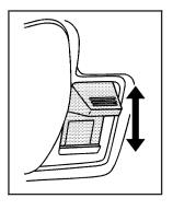
Lock and unlock the door from the outside using the key or the RKE transmitter, if available. From the inside, slide the manual lever on the door up or down.
