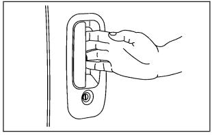
To open the front portion of a 60/40 door from the outside, pull out on the handle and open the door.
