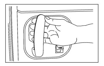
To open the sliding side door from the inside, pull the handle toward the rear of the vehicle. Then, slide the door toward the rear of the vehicle.
