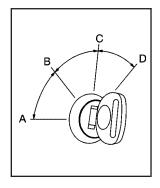
The ignition switch has four different positions.
