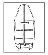
If the position you are using has an integrated headrest or head restraint and you are using a single tether, route the tether over the headrest or head restraint.
