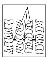
One way to tell when it is time for new tires is to check the treadwear indicators, which appear when your tires have only 1/16 inch (1.6 mm) or less of tread remaining.
