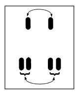
If the vehicle has dual rear wheels and the tread design for the front tires is different from the dual rear tires, always use the correct rotation pattern shown here when rotating the tires. The dual tires are rotated as a pair and the inside rear tires become the outside rear tires.
