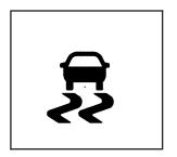
Press and hold the StabiliTrak button located on the instrument panel for more than five seconds to turn off StabiliTrak and part of the traction control system.
