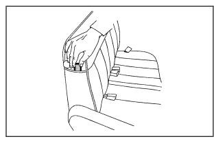
Locate the guide in a pocket on the side of the seatback.
