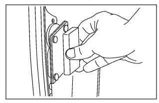
To open the driver side rear door, pull the latch release at the inside edge of the door.
