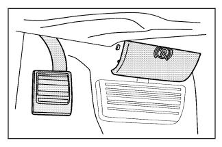
To set the parking brake, hold the regular brake pedal, then push down the parking brake pedal.
