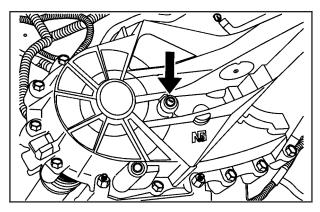
If the level is below the bottom of the filler plug hole, you'll need to add some lubricant. Add enough lubricant to raise the level to the bottom of the filler plug hole. Use care not to overtighten the plug.
