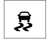
The StabiliTrak light comes on the instrument panel cluster when the system is turned off or requires service.
