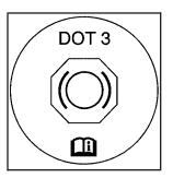
The brake master cylinder reservoir is filled with DOT 3 brake fluid. See Engine Compartment Overview on page 6-14 for the location of the reservoir.
