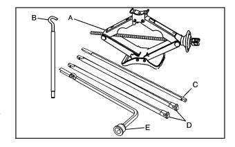
**Front Flat:** Assemble the jack (A) together with the jack handle (B), 1 or 2 jack handle extensions (D) and the wheel wrench (E).
