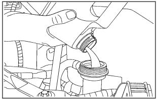
3. Fill the radiator with the proper DEX-COOL® coolant mixture, up to the base of the filler neck. See *Engine Coolant on page 6-28* for more information about the proper coolant mixture.
