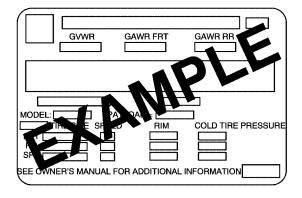
A vehicle specific Certification/Tire label is found on the rear edge of the driver door. The label shows the size of your vehicle's original tires and the inflation pressures needed to obtain the gross weight capacity of your vehicle.
