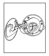
The tethered fuel cap is located behind a hinged fuel door on the driver side of the vehicle.
