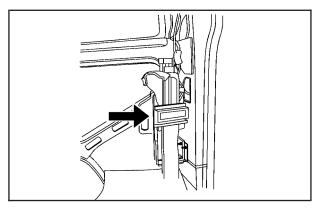
Remove the retaining wing bolt and lift it off of the mounting bracket.
