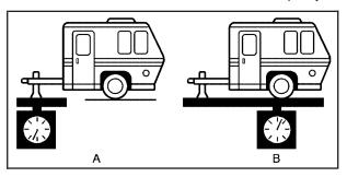
The trailer tongue weight (A) should be 10 percent to 15 percent of the total loaded trailer weight (B), up to a maximum of 400 lbs (181 kg) with a weight carrying hitch. The trailer tongue weight (A) should be 10 percent to 15 percent of the total loaded trailer weight (B), up to a maximum of 1,000 lbs (454 kg) with a weight distributing hitch.
