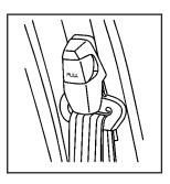
To move it down, pull on the center adjuster control labeled PULL. You can move the height adjuster up just by pushing up on the shoulder belt guide.
