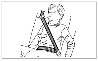
Buckle, position, and release the safety belt as described in previously in this section. Make sure that the shoulder belt crosses the shoulder.
