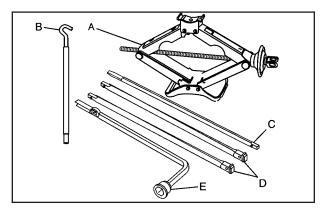
The tools you will be using include the jack (A), jack handle (B), hoist extension (C), jack handle extension (D), and the wheel wrench (E).
