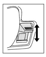
To lock the door from the inside, slide the manual lever on the door down. To unlock the door, slide the manual lever up.
