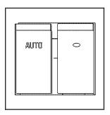
If the vehicle has power windows, the controls are located on each of the side doors. The driver door also has a control to operate the front passenger window.
