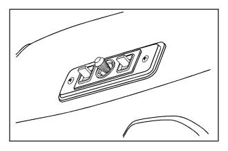
If the vehicle has front power seat(s), the controls are located at the front center of the seat cushion.
