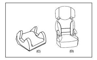
A booster seat (C-D) is a child restraint designed to improve the fit of the vehicle's safety belt system. A booster seat can also help a child to see out the window.
