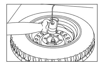
When the tire has been lowered, pull the tire toward you so you can reach the tire retainer and pull it up through the wheel opening.
