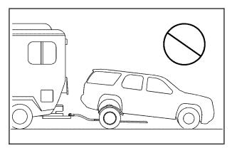
The vehicle was not designed to be towed with two wheels on the ground. To properly tow these vehicles, they should be placed on a platform trailer with all four wheels off the ground.
