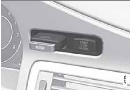
Ignition switch with remote key inserted (see page 77 for more information on ignition modes)
