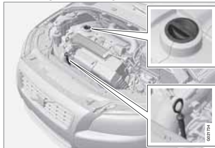
Location of the filler cap and dipstick
