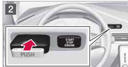
Ignition switch with remote key inserted (see page 77 for more information on ignition modes)
