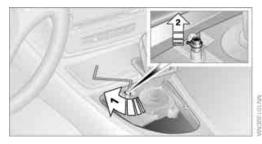
Insert allen wrench into the opening, arrow 1.
