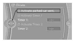
The parked car ventilation is switched on. Section 2.1 The symbol on the automatic climate control display flashes.
