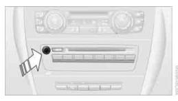
Press the button if the sound output is switched off.
