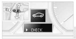
Push button 1 in the turn signal/high beam lever up or down repeatedly until the appropriate symbol appears in the display, accompanied by the words "CHECK". 2. Press button 2.
