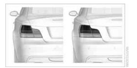
On the left: normal braking. On the right: sharp braking.
