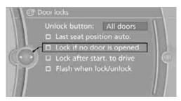
The function is switched on and is stored for the remote control currently in use.
