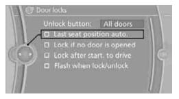
The function for automatically calling up the last seat position is switched on and is stored for the remote control currently in use.
