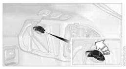
The outer brake lamp can be accessed through a single socket.
