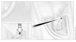
3. Using the screwdriver from the onboard vehicle tool kit, refer to page 213, press the red lever, see arrow, while moving the selector lever to the desired position.
