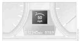
When the speed at which the vehicle is traveling is stored or when a stored speed is called up, the speed is briefly displayed in the instrument cluster.
