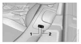
To move the front seats forward or backward from outside or from one of the rear seats: with the door open, press the front end **1** or rear end **2** of the switch.
