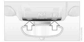
2. On both sides, use the screwdriver to press on the clip inside the opening.
