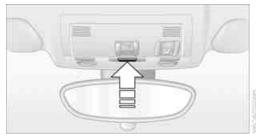
Interior lamps, front and rear\*: To switch on and off, press the button.
