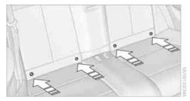
The anchor points for the lower LATCH anchors are located at the positions indicated by arrows, in the gap between the seat and the backrest.
