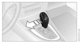
Push selector lever toward the left from the selector lever position D, the Sport program is activated. This position is recommended for a performance-oriented driving style.
