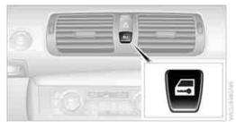
This button serves to unlock or lock doors and the trunk lid, but does not activate the anti-theft system. The fuel filler flap remains unlocked.
