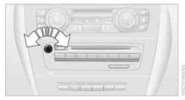
Turn the knob until the desired volume is set. Adjusting the volume for:
