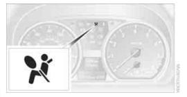
As of radio readiness, refer to page 55, the warning lamp comes on briefly to indicate that the entire airbag system and the belt tensioners are operational.
