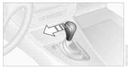
Move selector lever from position D toward the left into the M/S shifting slot; the Sport program is activated. This position is recommended for a performance-oriented driving style.
