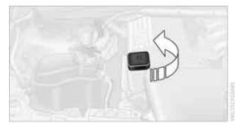
Do not add 1 US quart/1 liter of engine oil until a corresponding message is shown on the Control Display. Add oil within the next 125 miles/200 km; otherwise, the engine could be damaged.◀
