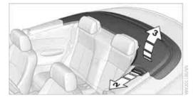
3. The locking pins must have engaged completely. If they are still visible: close the convertible top box cover as far as necessary until the locking bolts engage audibly, then slowly open the cover. During this process, do not close the convertible top box cover completely.
