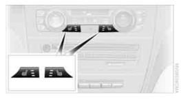
Press the button once per temperature level. Three LEDs indicate the highest temperature.
