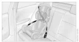
The rear safety belts and the front passenger safety belt can be prevented from being pulled out in order to fasten child restraint systems.
