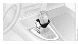
Using the allen wrench from the toolkit, refer to page 213, rotate the cover until it reaches the stop, arrow 1, and remove, arrow 2.
