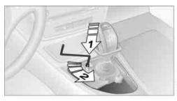
5. Rotate allen wrench until it reaches the stop, arrow **2**. The parking lock is unlocked.
