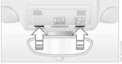
There are reading lamps at the front and rear\*, next to the interior lamps. To switch on and off, press the button.
