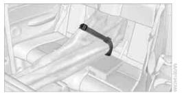
After loading, secure the transport bag and its contents. Tighten the retaining strap on the tensioning buckle for this purpose.
