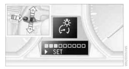
Push button 1 in the turn signal/high beam lever up or down repeatedly until the appropriate symbol appears in the display, accompanied by the brightness level and the word "SET".
