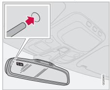
The upper left-hand corner of the rearview mirror has an integrated display that shows the compass direction toward which the car is pointing. Eight different directions can be displayed: N, NE, E, SE, S, SW, W and NW. The display shows your car's orientation with respect to true north.
