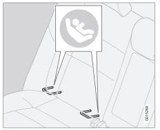
ISOFIX/LATCH lower child restraint anchors
