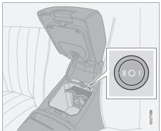
The refrigerator is located under the cover in the front seat center armrest. Use the button (see the inset illustration) to adjust the level of cooling.
