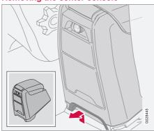
In order to make it possible to move the center seat in the second row of seats as far forward as possible (seven-seat models only), the rear section of the center console can be removed.
