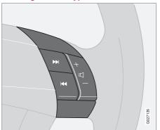
The four buttons on the steering wheel keypad can be used to control the audio system. The steering wheel keypad can be used to adjust volume, shift between preset stations and change CD tracks.
