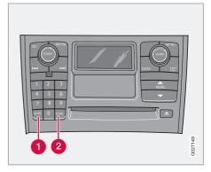
This function automatically searches for, and stores up to 10 strong AM or FM stations in a separate memory. If more than 10 stations are found, the 10 strongest ones will be stored. The function is especially useful in areas in which you are not acquainted with radio stations or their frequencies.
