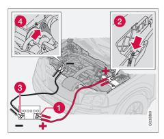
Follow these instructions to jump start your vehicle's dead battery or to jump start another vehicle's dead battery using your vehicle. Although your vehicle's battery is located under the floor of the cargo area, jumper cables should be connected in the **engine compartment**, to the points shown in the illustrations.
