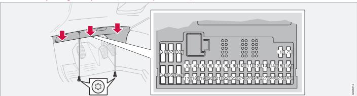
This fuse box is located behind the plastic cover below the steering wheel. When replacing a blown fuse, be sure to replace it with a new one of the same color and amperage (written on the fuse).
