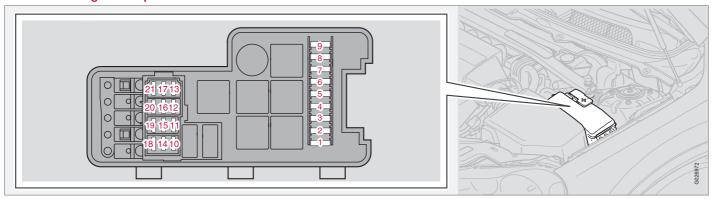
When replacing fuses, be sure to replace a blown fuse with a new one of the same color and amperage (written on the fuse).
