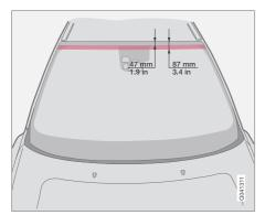
Section of the windshield where the IR-coating is not applied
