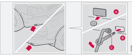
Positions for attaching towing eyelets
