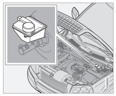
The brake fluid should always be above the MIN mark on the side of the reservoir. Check, without removing the cap, that there is sufficient fluid in the reservoir.
