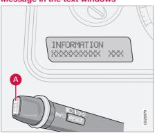
When a warning light in the instrument panel comes on, a message is also displayed in the text window. After you have read the message, you can erase it by pressing button A (see illustration).
