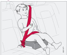
Volvo's own integrated booster cushion has been specially designed to help safeguard a child seated in the rear seat. When using an integrated booster cushion, the child must be secured with the vehicle's three-point seat belt.
