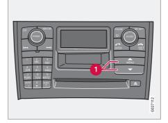
In menu mode, you can change settings and program new functions in the audio system. The various menu alternatives are shown in the display, and the current level in the menu structure is shown at the upper right corner of the display.
