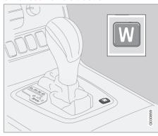
Press the **W** button at the base of the gear selector to engage/disengage this driving mode (see illustration). The **W** symbol will appear in the display (see page 58) when the function is activated.
