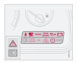
This shows that the symbols are functioning. When the engine starts, all symbols go out. If the engine is not started within 5 seconds, all symbols except **CHECK ENGINE** and go out. Certain symbols may not have their functions illustrated, depending on the vehicle's equipment. The symbol for the parking brake goes out when the parking brake is released.
