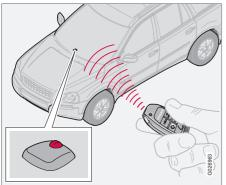
Your vehicle is equipped with two coded remote key transmitters with integrated ignition keys called Key Integrated Remote (KIR).
