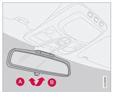
To reduce glare from the headlights of following vehicles, use the control to switch between the normal and night-driving positions.
