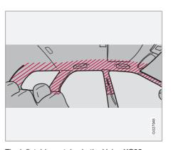
The inflatable curtains in the Volvo XC90 are also designed to help protect the occupants of the vehicle in a roll-over situation, and to help prevent them from being thrown from the vehicle if a roll-over occurs.
