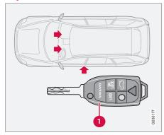
Your vehicle is equipped with two coded remote key transmitters with integrated ignition key blades called Key Integrated Remote (KIR).
