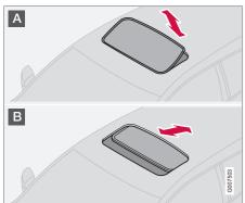
To operate the moonroof, turn the ignition key to position I or II, or start the engine. The moonroof can be operated in two ways:
