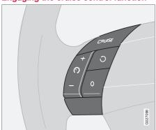
The cruise control panel is located on the left side of the steering wheel hub.
