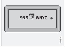
Example of an HD Radio station with sub-channels
