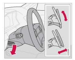
Both the height and the reach of the steering wheel can be adjusted to a comfortable position for the driver. Pull down the lever on the left of the steering column. Adjust the steering wheel to a suitable position and press the lever back into place to lock the steering wheel in the new position. Check that the steering wheel is locked in the new position.
