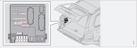
The fuses in the cargo area are located behind the panel on the driver's side of the cargo compartment. When replacing a blown fuse, be sure to replace it with a new one of the same color and amperage (written on the fuse).
