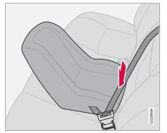
Pull out the shoulder section of the seat belt
