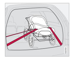
As a safety precaution, all cargo in your vehicle should be securely anchored to keep it from being thrown forward in the event of sudden braking, etc. The vehicle is equipped with eyelets in the cargo space to which straps or other cargo restraints can be attached.
