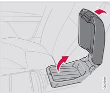
To open the lid on the storage compartment, press the lower edge of the opening latch (see illustration above). This lid can be folded back to form a small table area for rear seat passenaers.
