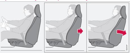
The Whiplash Protection System (WHIPS) consists of specially designed hinges and brackets on the front seat backrests designed to help absorb some of the energy generated in a collision from the rear (when the vehicle is "rearended").
