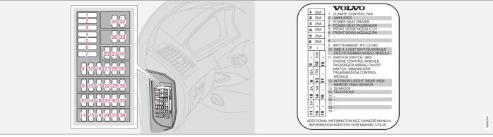
The decal shows the positions and amperage of the fuses
