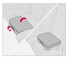
The booster cushion must be pressed down before the backrest can be folded down.
