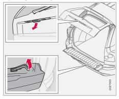
To open the upper section of the tailgate, pull the handle downward.
