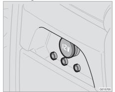
RSE-AUX connectors are located on the rear side of the tunnel console
