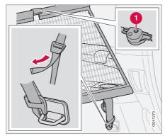
Folding and storing the cargo net Press the release buttons on the hinges (1 in the illustration) and fold the net.
