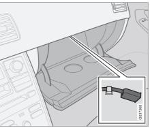
USB connector in glove compartment
