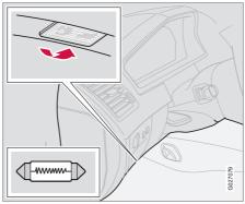
The door step courtesy lights are located under the dashboard on the driver's and passenger's sides.
