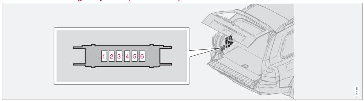
The fuses in the cargo area are located behind the panel on the driver's side of the cargo compartment. When replacing a blown fuse, be sure to replace it with a new one of the same color and amperage (written on the fuse).
