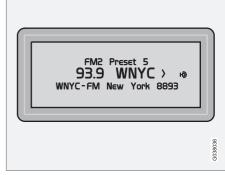
Display when the radio is receiving an HD Radio broadcast
