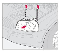
The entire lamp housing must be lifted out when replacing these bulbs.
