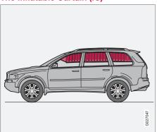
This system consists of inflatable curtains located along the sides of the roof liners, stretching from the front side windows to the rear edge of the rear side windows. It is designed to help protect the heads of the occupants of the front seats and the occupants of the outboard rear seating positions, including the outboard passenger in the third row of seats in certain side impact collisions.
