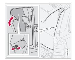
Move the catch rearward to unlock the fuel filler door lock, or move it forward to lock the filler door.
