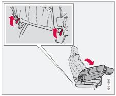
The front passenger seat backrest can be folded to a horizontal position to make room for a long load. Fold the backrest as follows:
