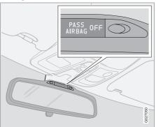
Occupant Weight Sensor (OWS) indicator light
