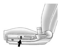
If available, press and hold the top or bottom of the switch to raise or lower the seat. Release the switch when the desired height is reached.
