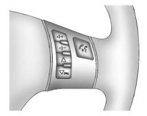
If equipped, some audio controls can be adjusted using the controls on the right side of the steering wheel.
