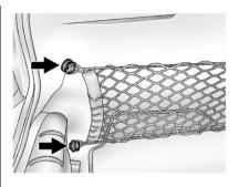
Remove the two rear convenience net hooks holding the trunk trim and move the trim aside.
