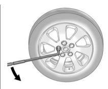
Use the wrench to loosen all the wheel nuts. Do not remove them yet.
