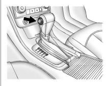
Press the + (plus) end of the button on the side of the shifter to upshift, or push the - (minus) end of the button to downshift.
