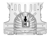
Turn the retainer clockwise and remove the tire sealant and compressor kit.
