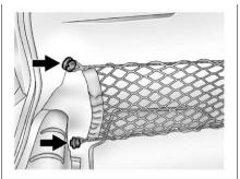
Remove the two rear convenience net hooks holding the trunk trim and move the trim aside.
