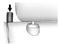
To lower the rear seatback, pull up on the seatback strap while folding the seatback down. This allows access to the trunk. To raise the rear seatback pull the seatback up and make sure it latches.
