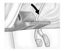
A driver side storage compartment is located near the steering column on the bottom of the instrument panel. Pull the cover down to open. Pull out to remove for cleaning.
