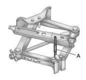
Place the jack over the bolt (A) on the floor, making sure it contacts the bolt. Thread the jack retainer nut until it contacts the jack.
