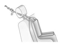
If the position you are using has an adjustable headrest or head restraint and you are using a dual tether route the tether under the headrest or head restraint and in between the headrest or head restraint posts. See Head Restraints on page 3-2.
