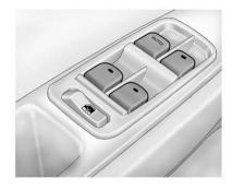
The power window switches are located on the armrest on the driver's door. In addition, there is a switch on each passenger door.
