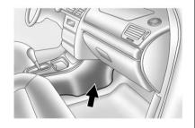
The instrument panel fuse block is located on the instrument panel near the floor on the passenger side of the vehicle.
