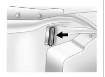
The rear compartment fuse block is located in the trunk of the vehicle. Access the fuse block through the trunk panel on the driver side of the rear cargo area.
