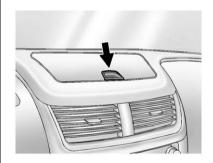
An instrument panel storage area, with a removable liner, is located above the radio. Slide the latch toward the rear of the vehicle to open the storage area.
