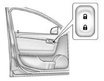
(Unlock): Press to unlock the doors.
