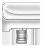
To set the parking brake, push down the parking brake pedal with your left foot. If the ignition is on, the brake system warning light will come on. See *Brake System Warning Light on page 5-17*.
