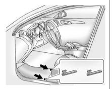
The driver side floor mat is held in place by two hooks.
