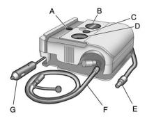
When using the tire sealant and compressor kit during cold temperatures, warm the kit in a heated environment for five minutes. This will help to inflate the tire faster.
