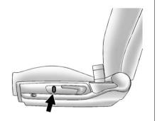
If available, press and hold the top or bottom of the switch to raise or lower the seat. Release the switch when the desired height is reached.
