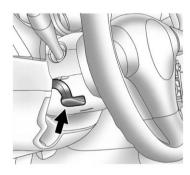
The lever is located on the left side of the steering wheel column.
