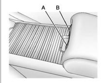
The center console storage has a tray and a main storage area. Pull up on the latch (A) to access the tray. Pull up on the latch (B) to access the main storage. It is equipped with a removable divider. There may be a storage pocket at the rear of the center console.
