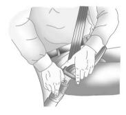
To unlatch the belt, push the button on the buckle. The belt should return to its stowed position. Slide the latch plate up the safety belt webbing when the safety belt is not in use. The latch plate should rest on the stitching on the safety belt, near the guide loop on the side wall.
