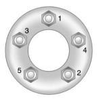
Tighten the wheel nuts firmly in a crisscross sequence, as shown, with the wheel wrench.
