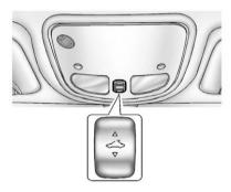
The sunroof only operates when the ignition is in ON/RUN or ACC/ACCESSORY, or if Retained Accessory Power (RAP) is active. See Retained Accessory Power (RAP) on page 9-18.
