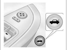
Press the button located on the driver door near the map pocket to open the trunk.
