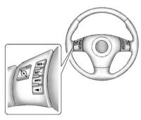
The cruise control buttons are located on the left side of the steering wheel.
