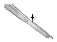
Extend the handle on the wheel wrench by pressing the button and pulling on the end of the wrench. You must do this before using the wheel wrench.
