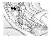
Press the + (plus) end of the button on the side of the shifter to upshift, or push the - (minus) end of the button to downshift. The Driver Information Center (DIC) in the instrument cluster will change from the currently displayed message to the letter "M," for Manual position, and a number indicating the requested gear.
