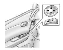
Controls for the outside power mirrors are located on the driver door.
