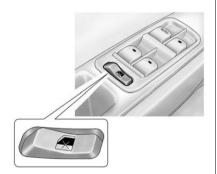
The rear window lockout switch is on the driver door. This feature prevents the rear passenger windows from operating, except from the driver position.
