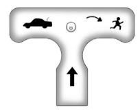
There is a glow-in-the-dark emergency trunk release handle located inside the trunk on the trunk latch. This handle glows following exposure to light. Pull the release handle up to open the trunk from the inside.
