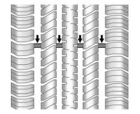
Treadwear indicators are one way to tell when it is time for new tires. Treadwear indicators appear when the tires have only 1.6 mm (1/16 in) or less of tread remaining. See *Tire Inspection on page 10-51* and *Tire Rotation on page 10-51* for more information.
