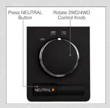
• When operating your vehicle in 4WD LOW, do not exceed 25 mph (40 km/h).
