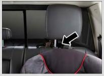
Tether Strap Through Outboard Tether Strap Loop
