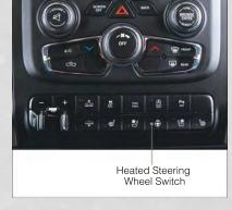
automatically shutting off. The heated steering wheel can shut off early or may not turn on when the steering wheel is already warm.
