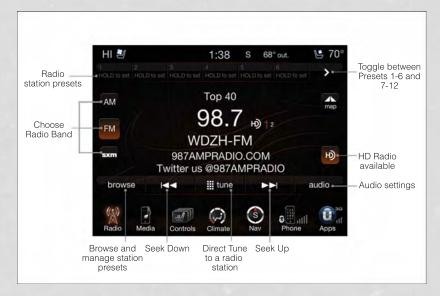
• To access the Radio mode, touch the Radio soft-key at the lower left of the screen.
