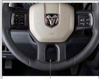
Hood Release (below steering wheel at base of instrument panel)
