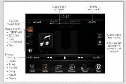
The iPod®/CD/AUX controls are accessed by touching the desired soft-key displayed on the side of the screen and choosing between Disc, AUX, iPod®, Bluetooth or SD Card.
