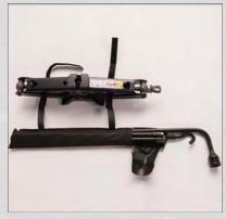
4. Place the jack and tools in the storage position holding the jack by the jack turn-screw, slip the jack and tools under the seat so that the bottom slot engages into the fastener on the floor.
