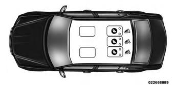
Lower Anchorage Symbol 2 anchorages per seating position
