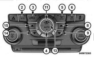
Automatic Climate Controls — Hard-keys (ATC System Shown)
