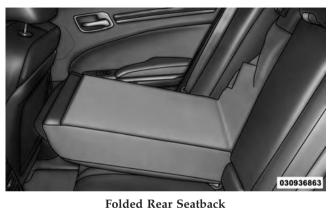
When the seatback is folded to the upright position, make sure it is latched by strongly pulling on the top of the seatback above the seat strap.
