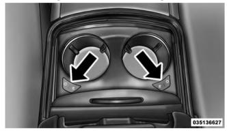
Heated And Cooled Cupholder Switches
