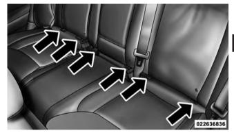
LATCH Anchorages Locating The LATCH Anchorages
