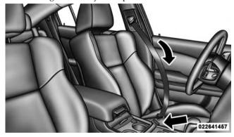
Pulling Out The Lap/Shoulder Belt Latch Plate
