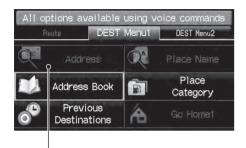
Certain manual functions are disabled or inoperable while the vehicle is in motion. You cannot select a grayedout option until the vehicle is stopped.
