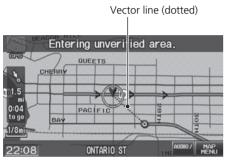
▶If Unverified Area Routing is Off, the route line uses verified streets only (when possible). A dotted "vector line" pointing directly towards your destination is also displayed.
