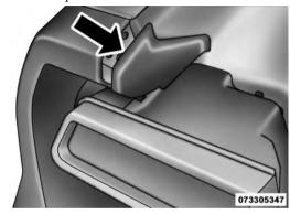
Reinstall Tail Lamp Retainer
