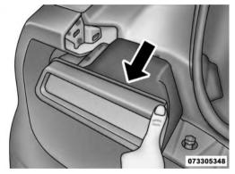
Removing Tail Lamp Assembly
