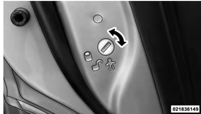
Child-Protection Door Lock Function
