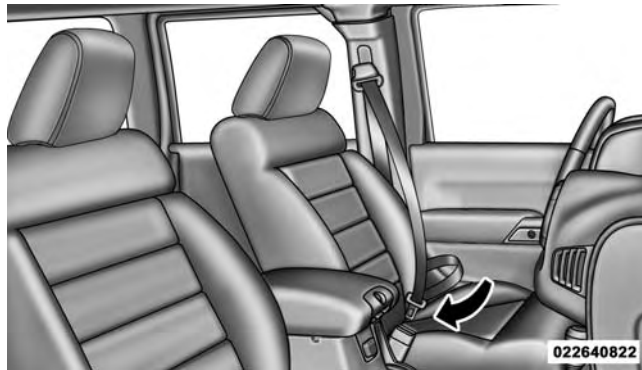
Inserting Latch Plate Into Buckle
