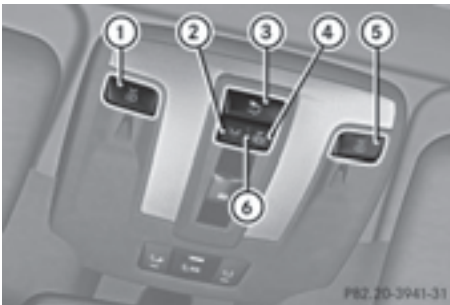
Front overhead control panel
